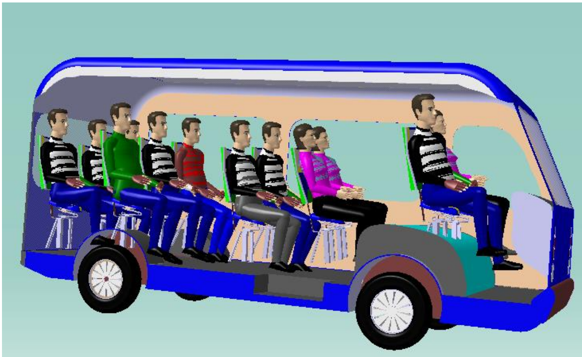
Figure 4. 41 Passenger seat layout with human body builder model
