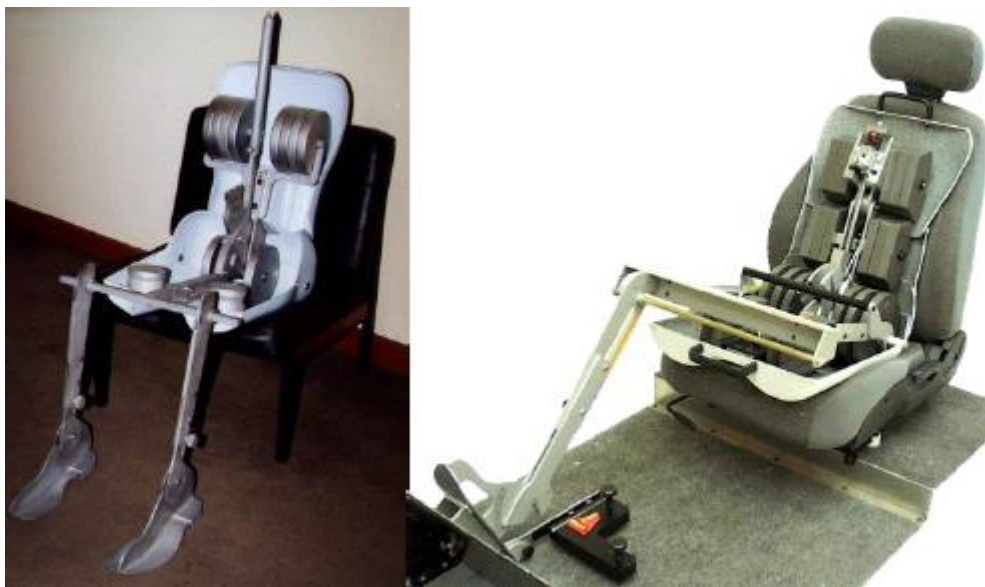
Figure 2. 4 Devices for measuring H-point, from SAE J826 and J4002
