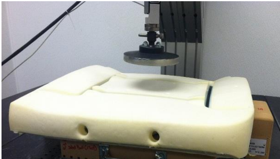
Figure 2. 2 IFD testing machine.
