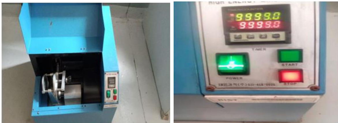
Figure 3.7 High energy ball milling machine for powder mixing process and
