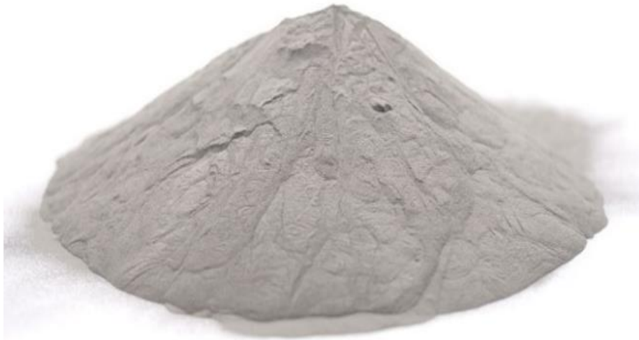
Figure 3.1 Titanium Ti-6AL- 4V powder
