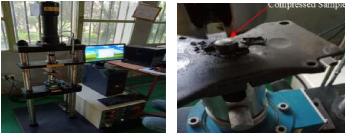
Figure 3.17 (A) UTM (Compression test) set up and (B) the compressed Sample)
