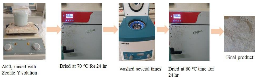
Figure 3. 4 Schematic representation of the preparation of Aluminum loaded zeolite Y
