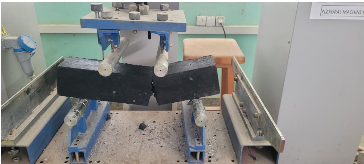
Appendix B3: Picture taken during beam flexural test
