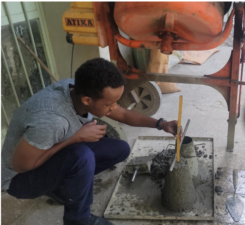
Figure 4.7 Performing slump test
