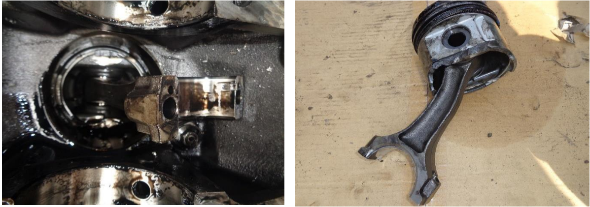
Figure C. 4. Engine connecting rod with piston where damage
