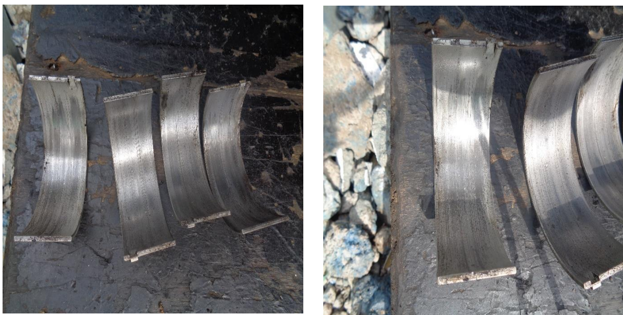
Figure C. 12. Engine bearing scratched and takes heat
