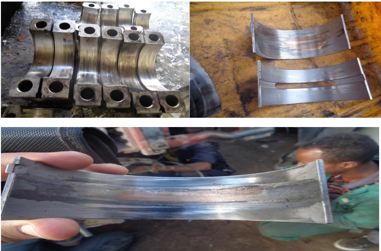
Figure C. 18. Engine main journal and con rod bearing scratched
