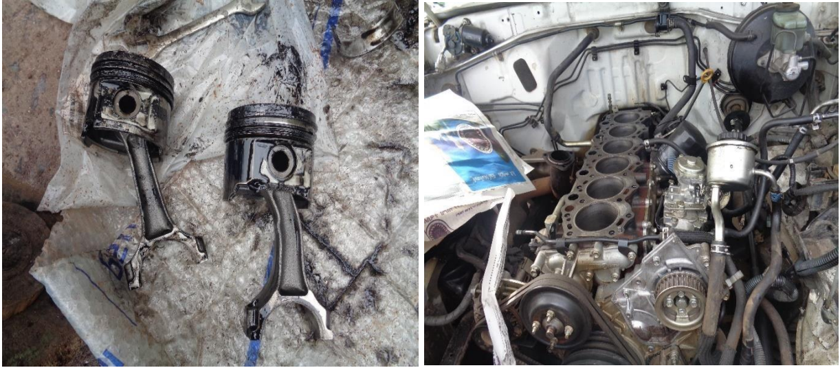
Figure C. 2. Engine internal parts connecting rod with piston damage
