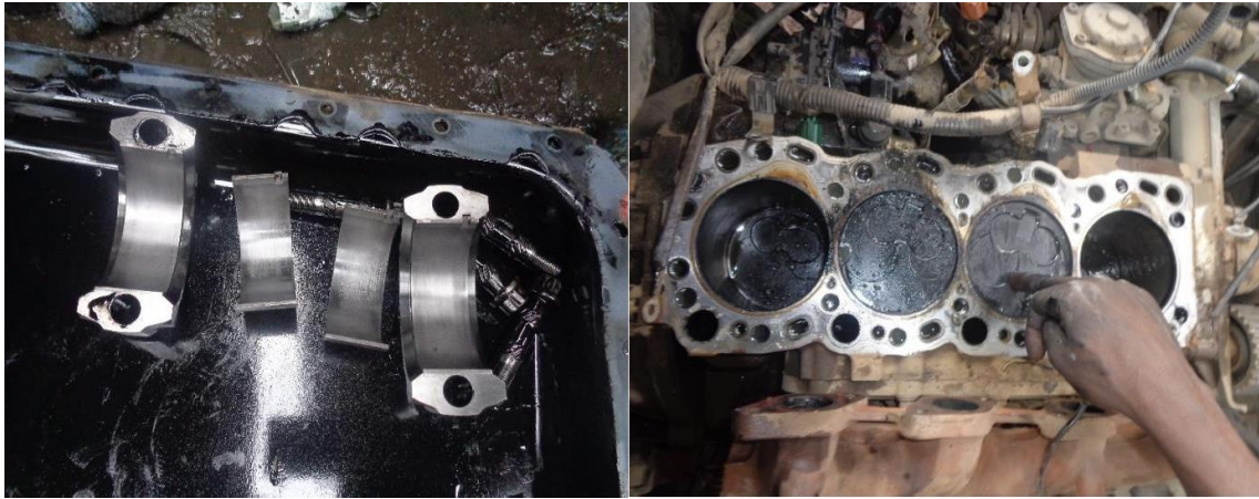
Figure C. 6. Engine cylinder head and bearing disassemble
