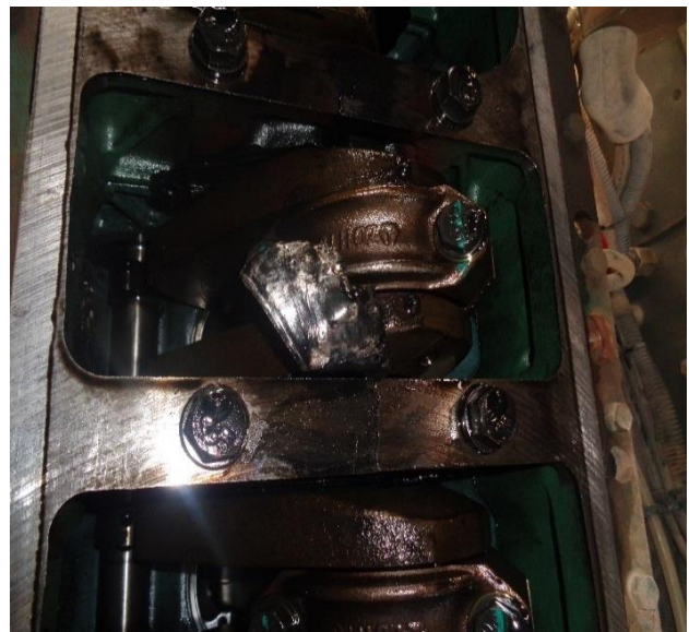
Figure C. 16. Engine crank shaft with shall bearing melted and damage
