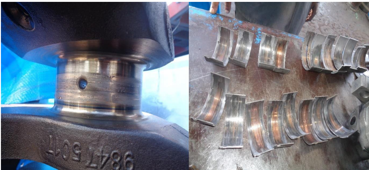
Figure C. 20. Engine main journal and con rod bearing stalled and takes heat
