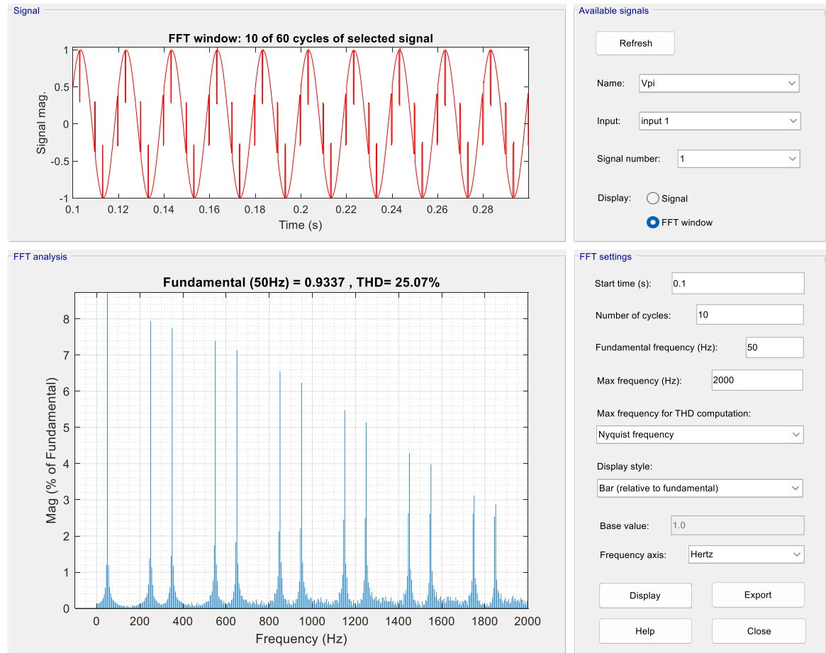
Figure 4.8. FFT analysis of the source voltage without DVR
