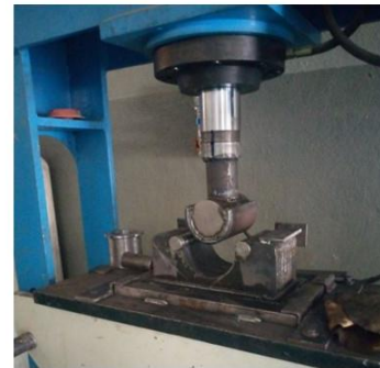
Figure 4.9 Mandrel diameter vs length of span with prepared jig
