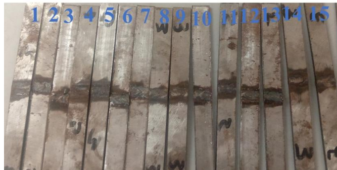
Figure 4.4 Hardness testing specimen prepared
