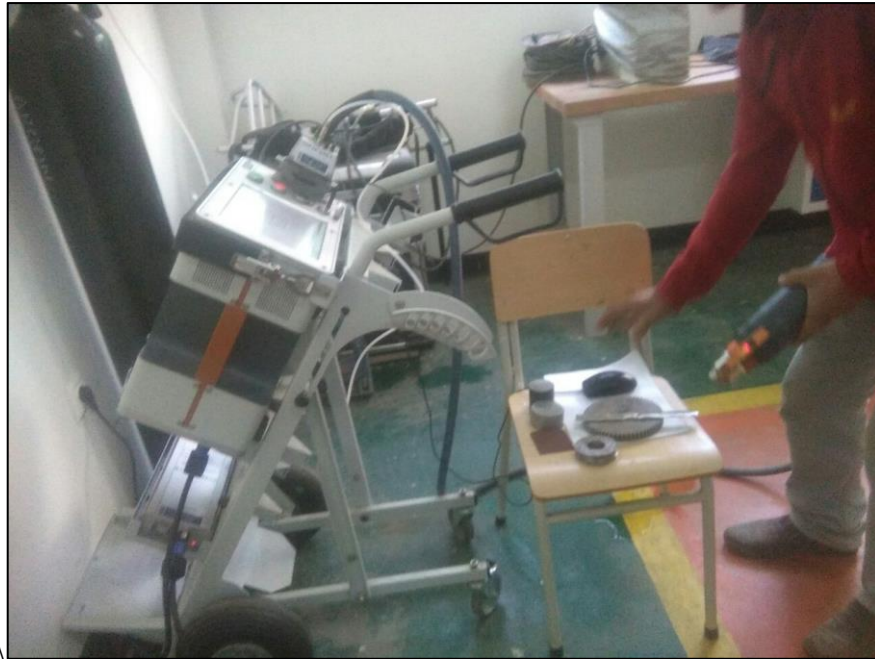
Figure 4.2 Composition analysis of AISI 4130 alloy steel through spectroscopy
