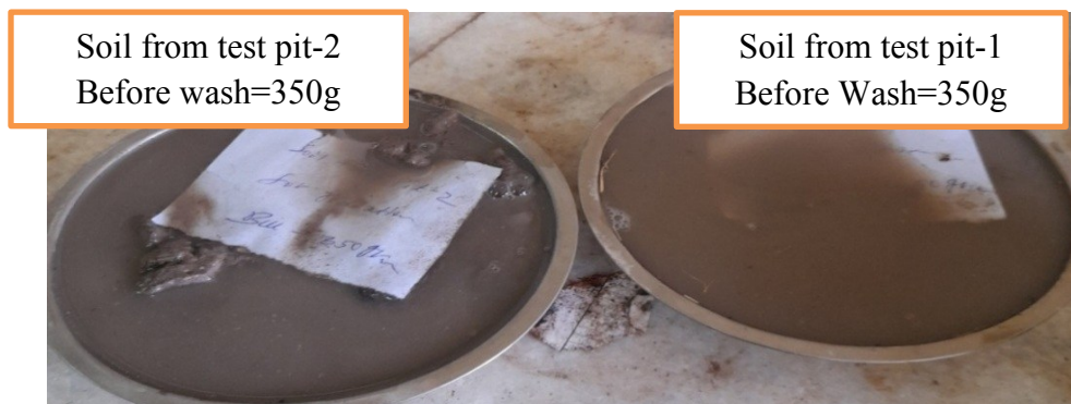
Figure 17: Soaked the soils in water for wet sieve analysis
