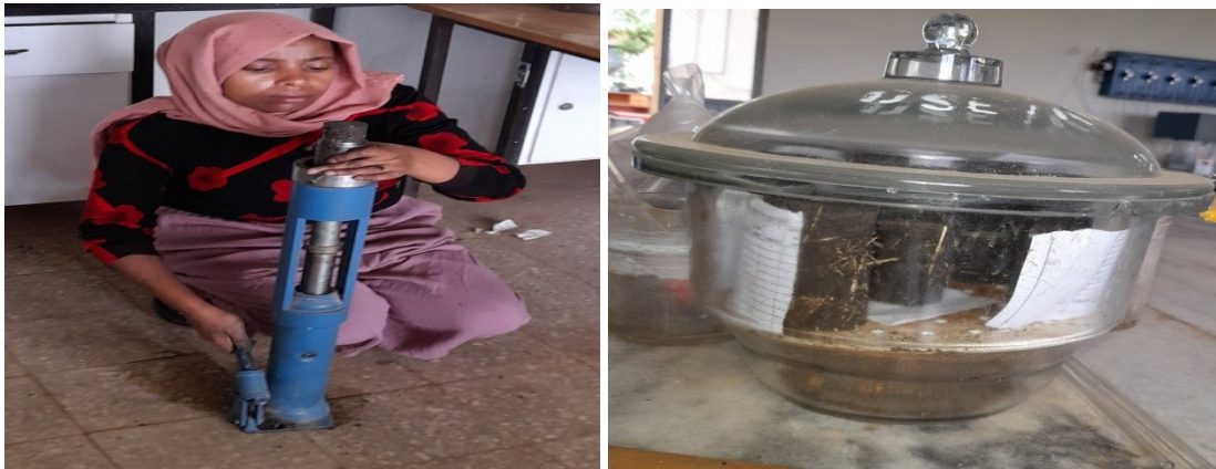
Figure 22: Sample preparation for unconfined compressive strength test
