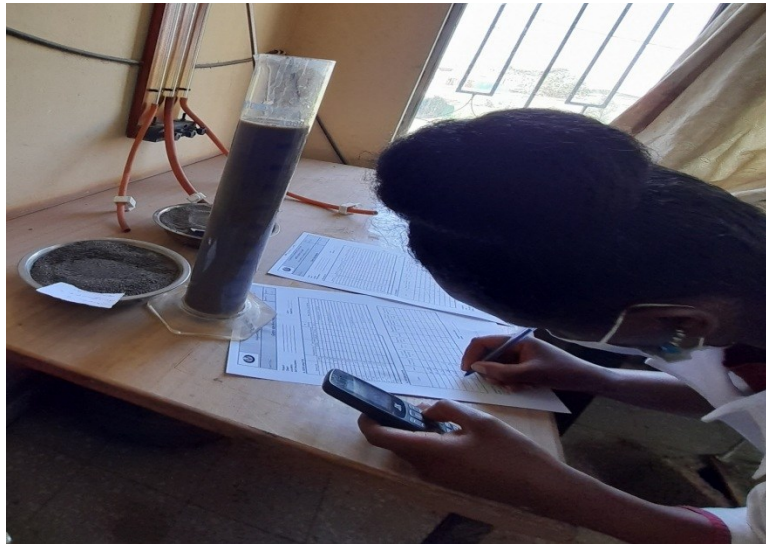
Figure 18: Recorded hydrometer floats in a slurry with the function of time
