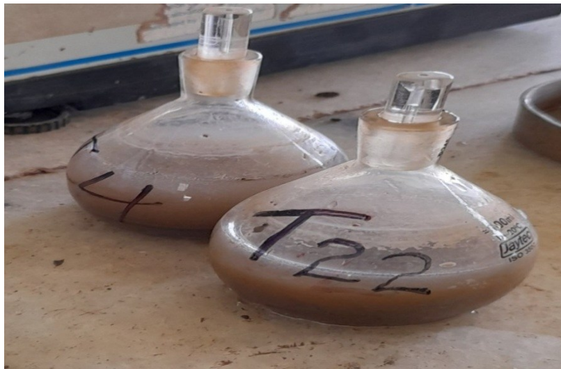
Figure 16: Specific gravity test for black cotton soil
