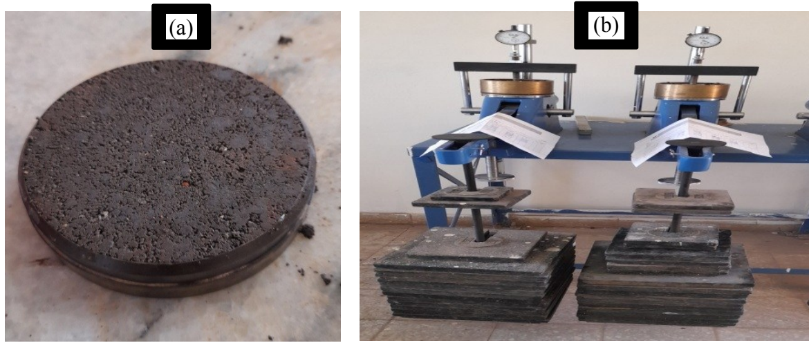
Figure 24: (a) Sample prepared for consolidation test (b) Consolidation test machine
