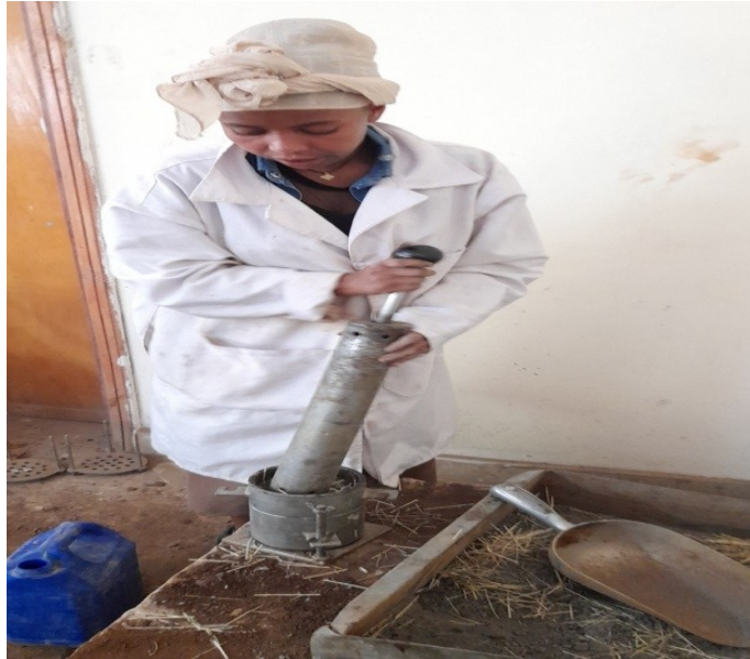
Figure 21: Standard compaction test
