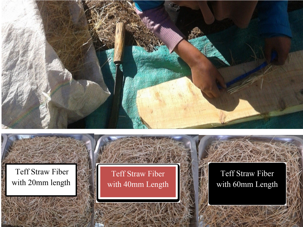
Figure 19: Prepared samples of teff straw fiber with different lengths
