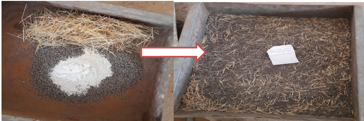
Figure 20: Prepared soil reinforced and lime stabilized sample for a compaction test
