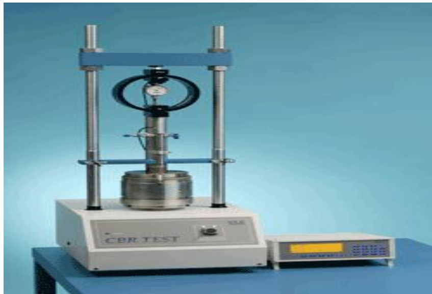
Figure 2.1 California bearing ratio device
