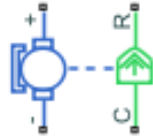
Figure C.4: DC Motor Block
