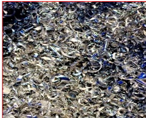
Figure 4.4 Chips generated during dry machining
