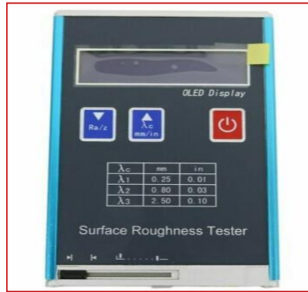
Figure 3.5 Surface roughness tester profilometer contact type
