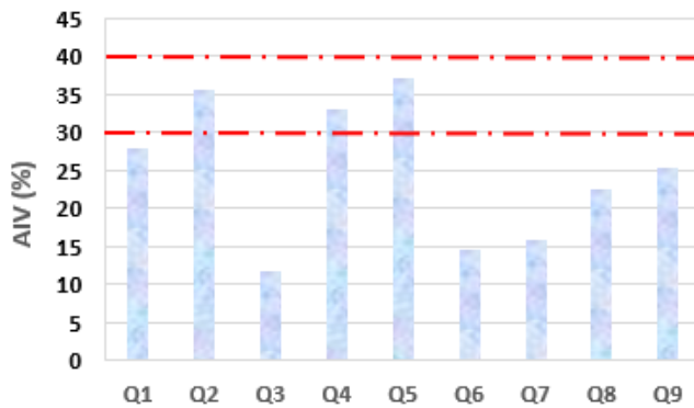
Figure 5.16: Aggregate impact value of the target areas
