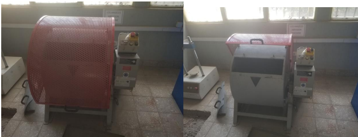
Figure 3.4: Los Angeles abrasion machine
