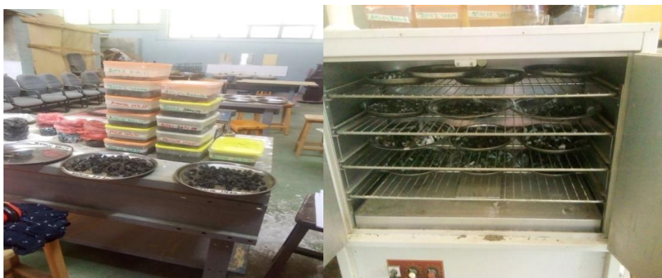
Figure 3.5: Immersion of the sample in sodium sulphate solution and oven drying phase
