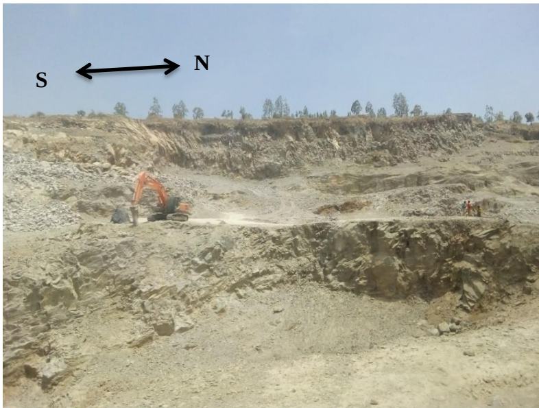
Figure 4.7: Existing quarry site of an ignimbrite outcrops in Adama town
