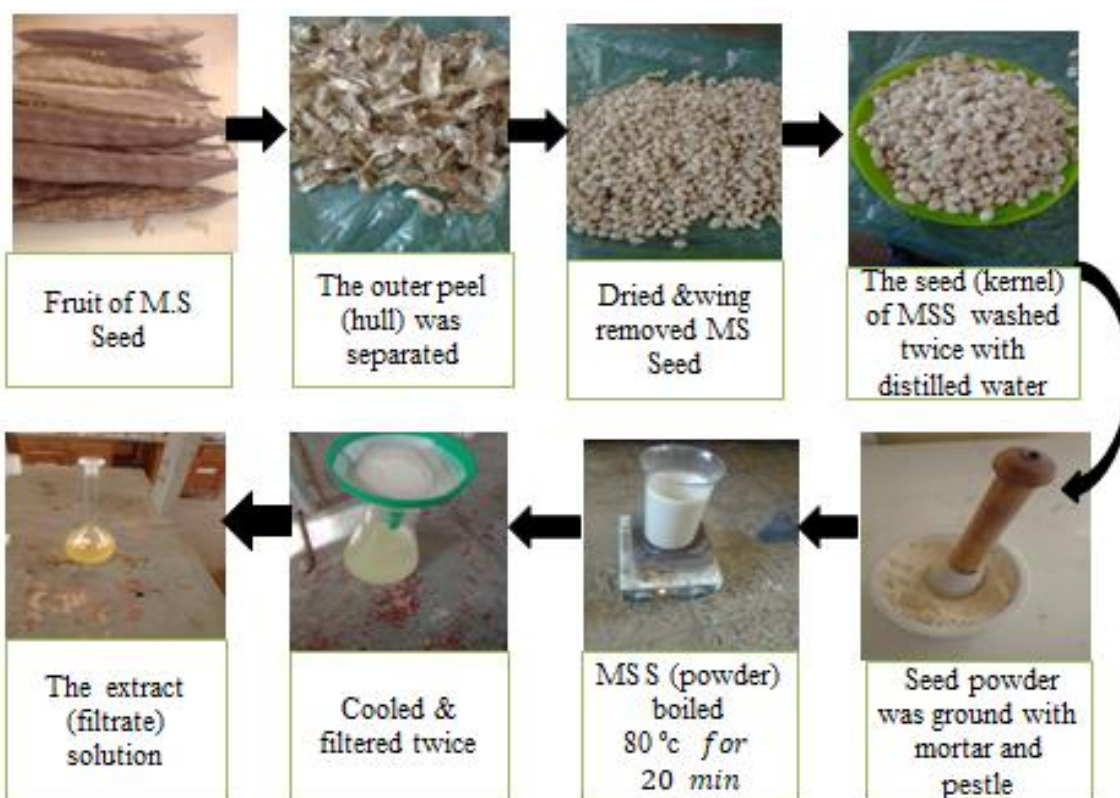
Figure : Flow diagram for the preparation of moringa stenopetala seed extract.
