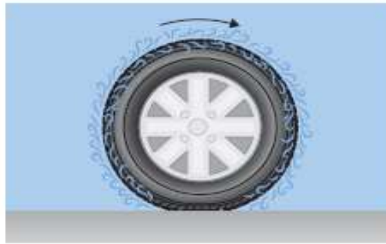
Figure 2.15: Aerodynamic drag of the rotating tyre
