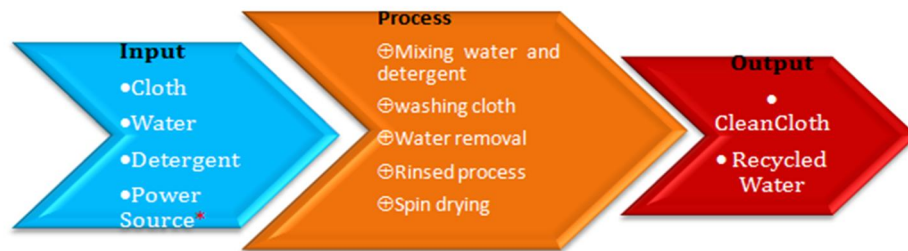
Figure 4:2 Function of the machine
