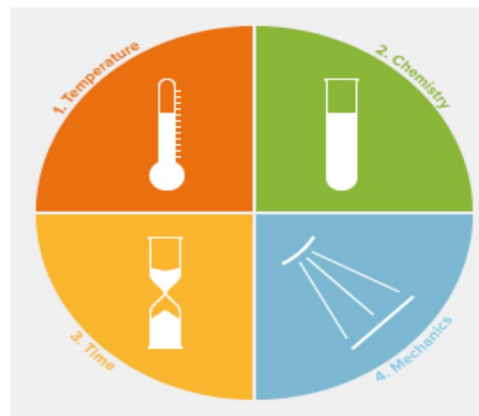
Figure 2:1 In washing machines the mechanical action is provided by the drum, agitator or impeller movement Source: based on glasswashing.biz 2012
