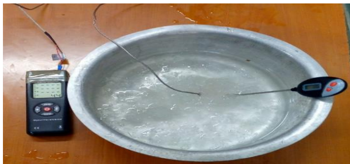
Figure 5.6 Calibration temperature measuring instrument with ice.
