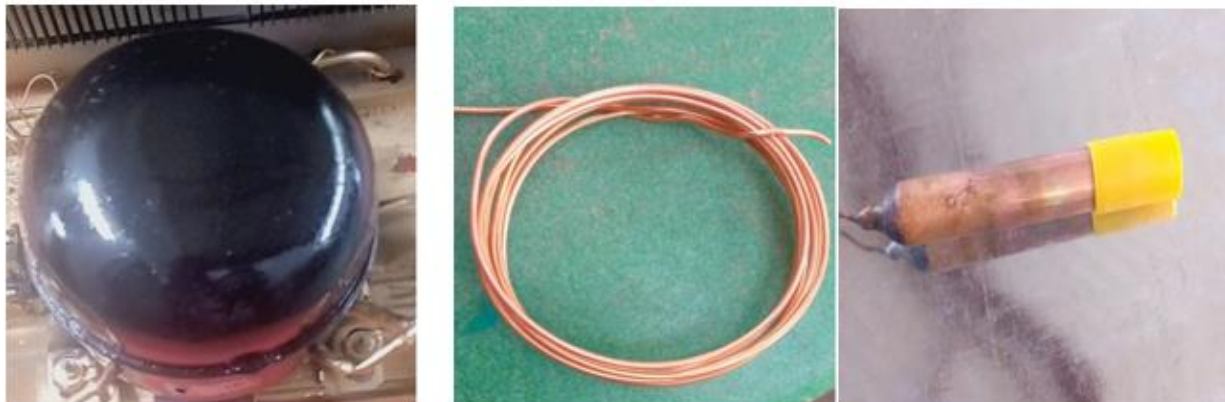
Figure 5.3 Compressor, capillary tube and filter drier.
