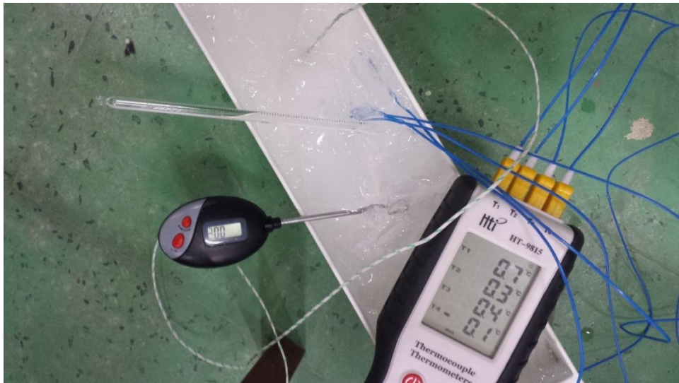
Figure 4.12: Calibration of temperature measuring instrument with ice bath
