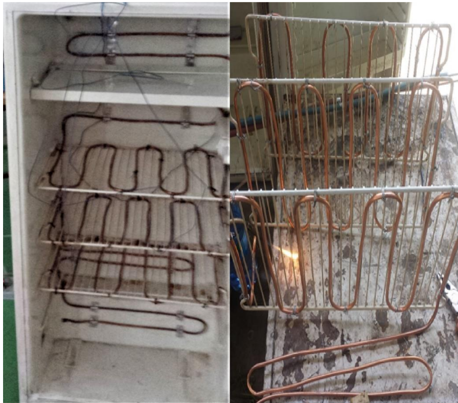
Figure 4.3: Evaporator installation on the refrigerator
