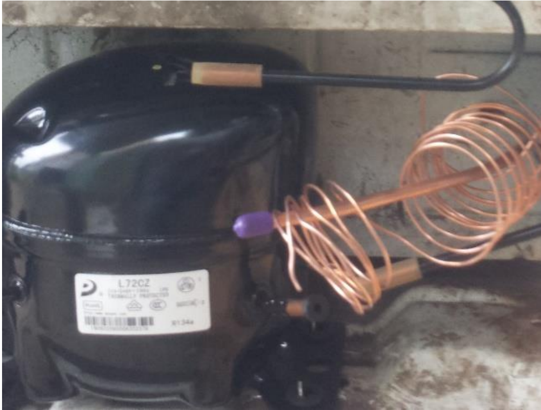
Figure 4.4: Placement of compressor on the refrigerator
