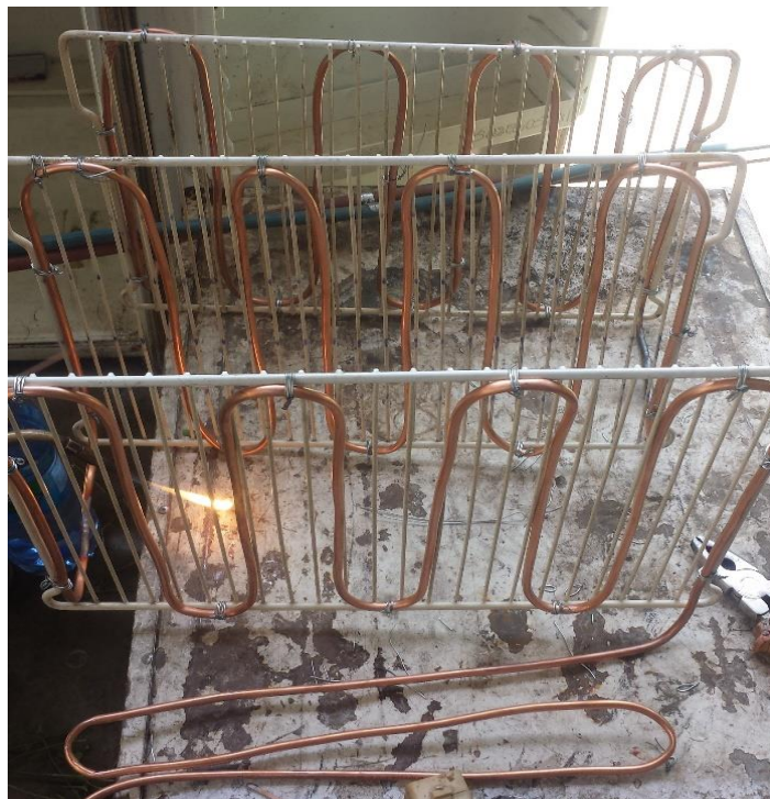
Figure 4.1: Fabrication of evaporator
