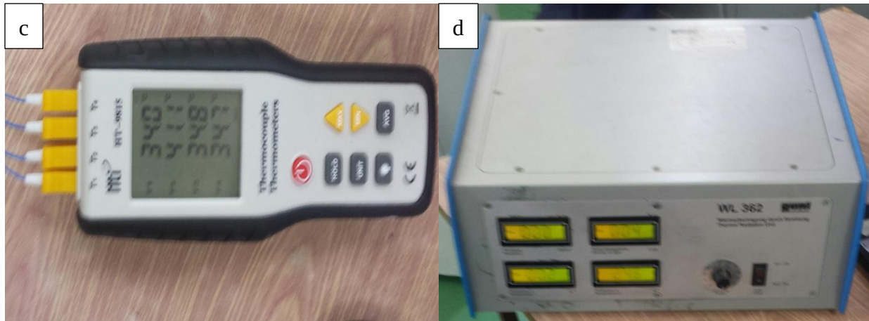
Figure 4.11: Temperature measuring instruments: (a) Digital thermocouple thermometer, (b) mercury thermometer (c) k type thermocouple (HT-9815) (d) k type thermocouple thermometer (WL-362),.
