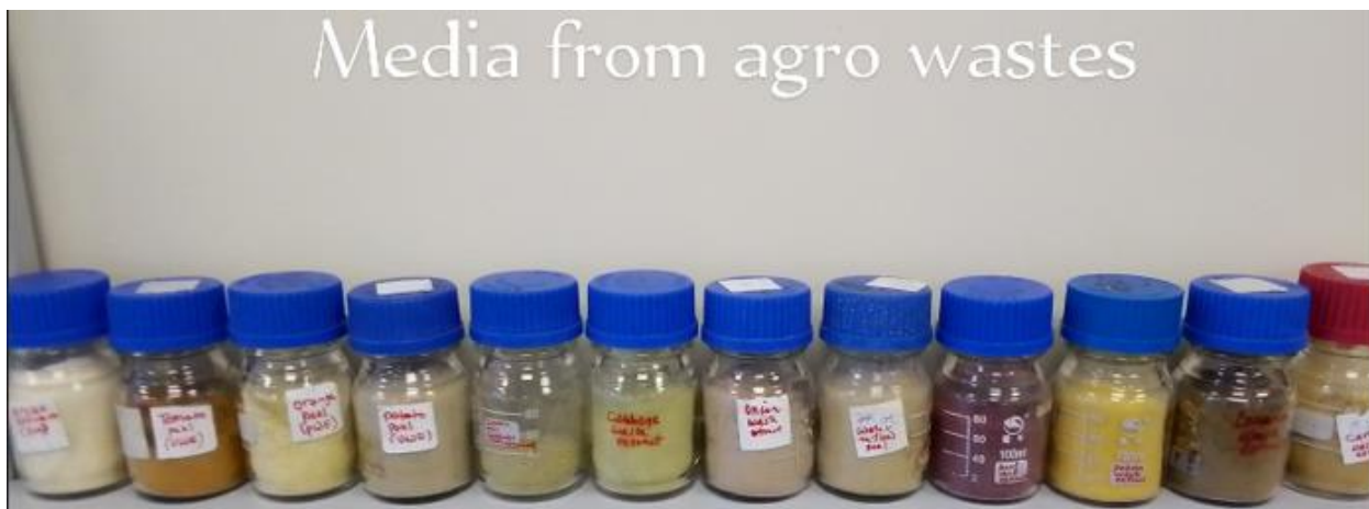
Figure 3 Media prepared from agro-waste residues to be used as alternative low-cost growth substrate
