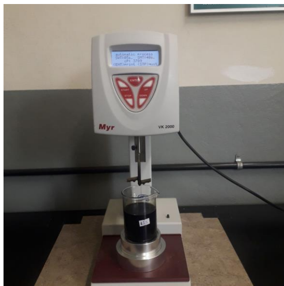
Figure 10 Viscosity measuring device ( Viscometer)
