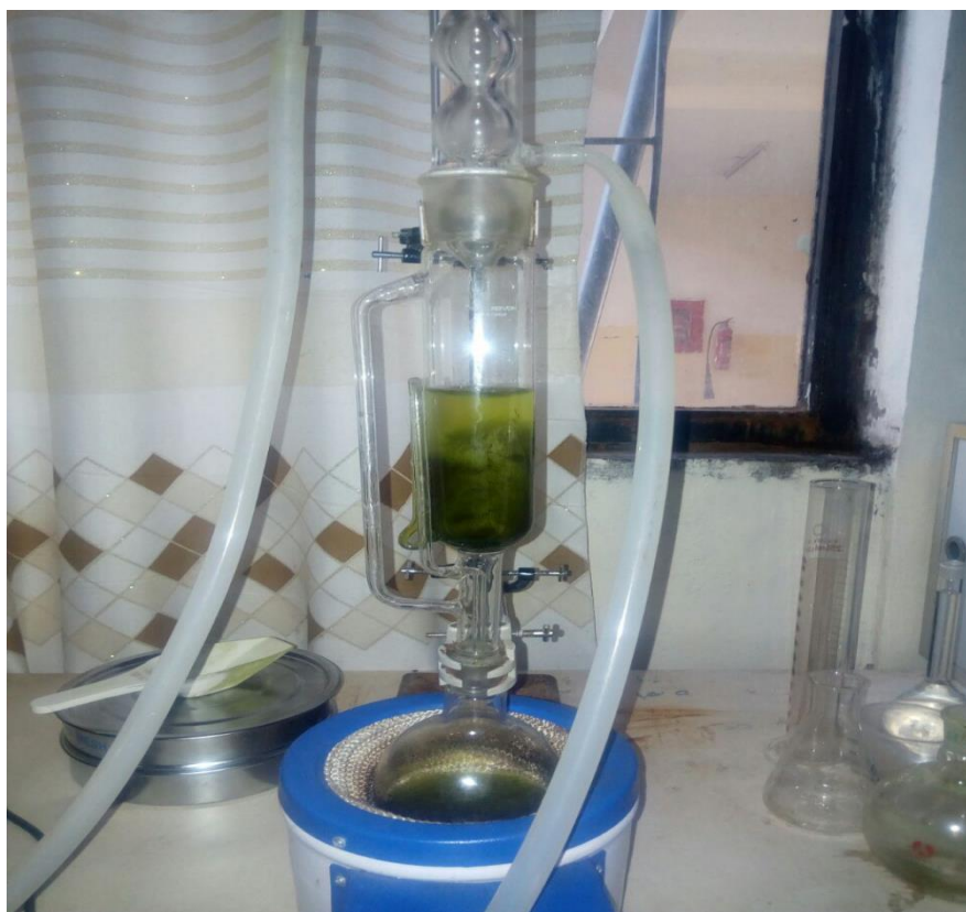
Figure-8 Soxhlet extraction set up
