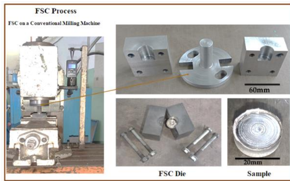
Figure 4.20 FSC Process on a Conventional Milling Machine
