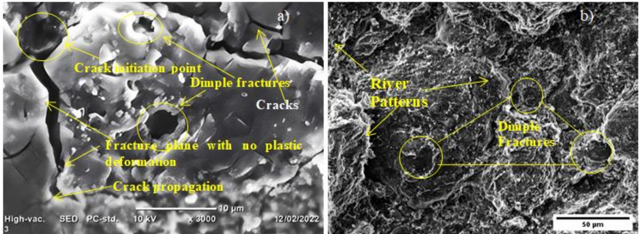
Figure 4. 5 SEM Fractography Observation of S-3 A) Longitudinal Surface B) Cross-Sectioned Surface
