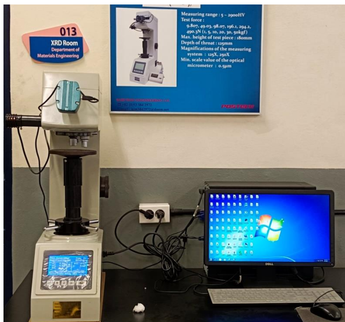
Figure VIII Hardness property testing machine
