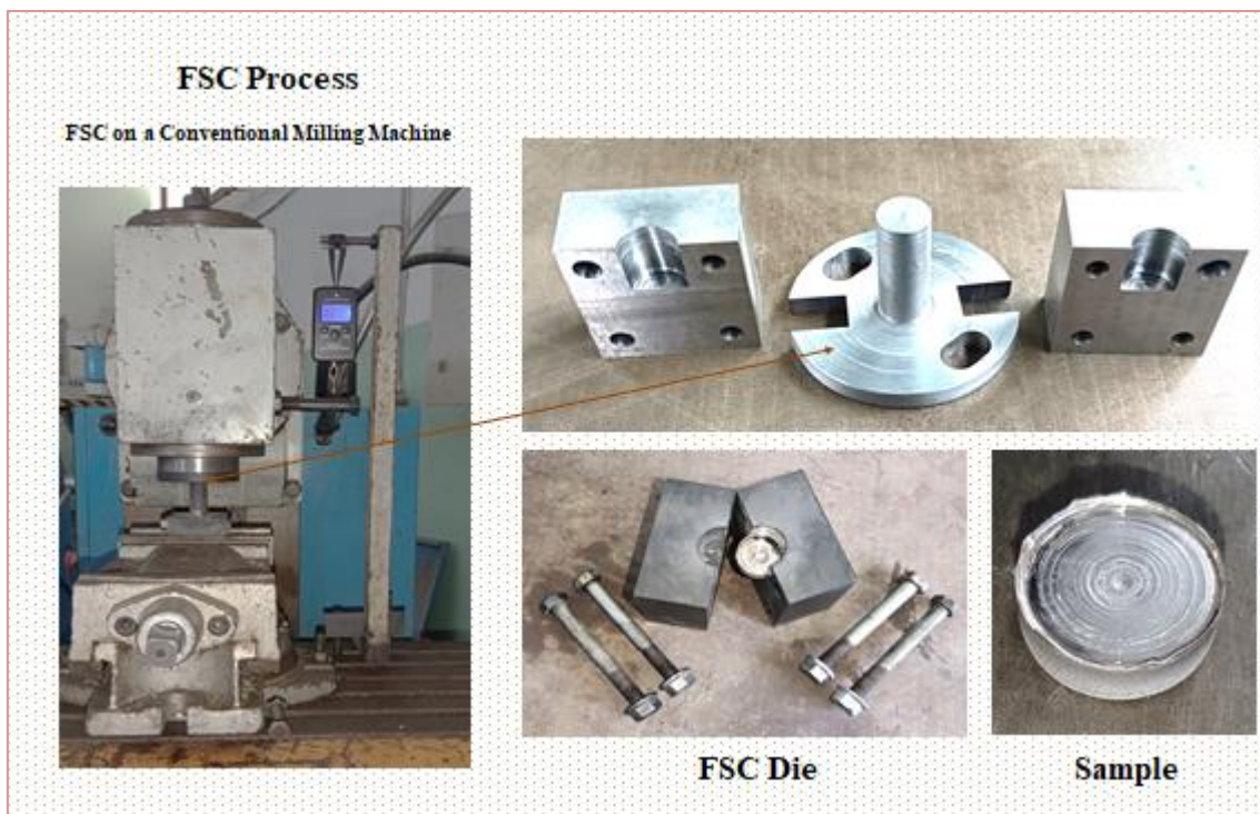
Figure IV FSC experimental setup and procedure on a conventional milling machine
