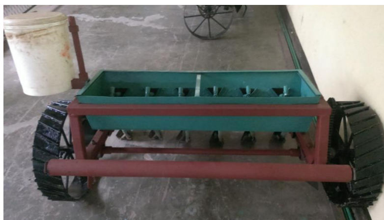
Fig: 3.20. Fabrication pictures of 2WT seed drill
