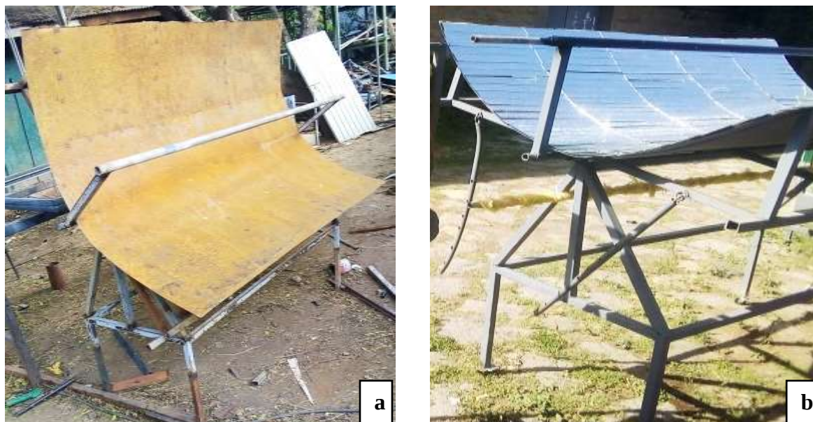
Figure 5.5 Preparation of parabolic trough solar collector a) without glass cover, b) with glass cover and tracking system
