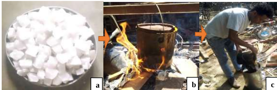
Figure 5.2 Preparation of phase change materials a) sizing the PCM, b) melting, c) filling
