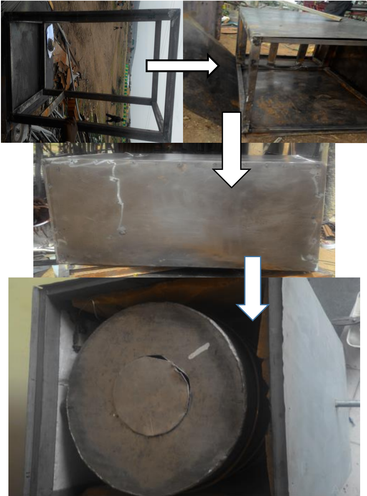
Figure 5.2: Manufacturing process of cooler box
