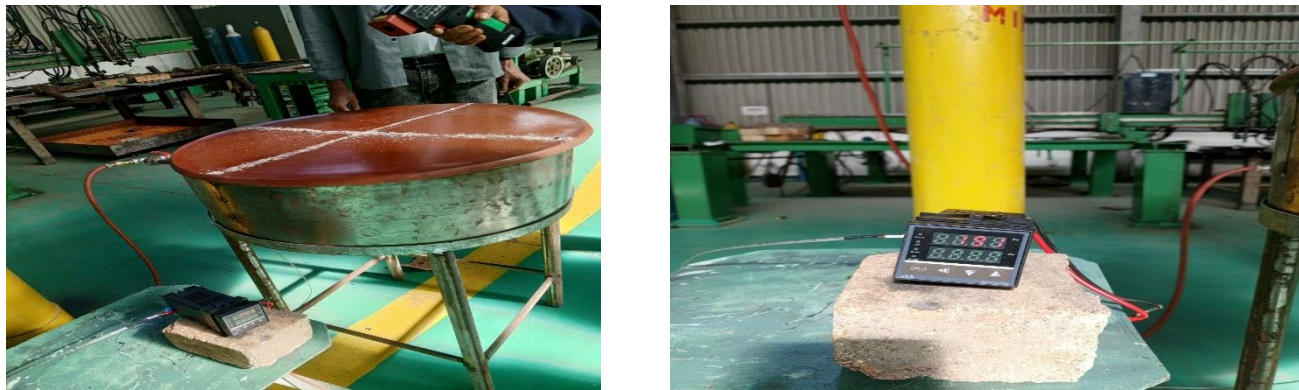
Figure 6.6 Combustion Temperature recording
