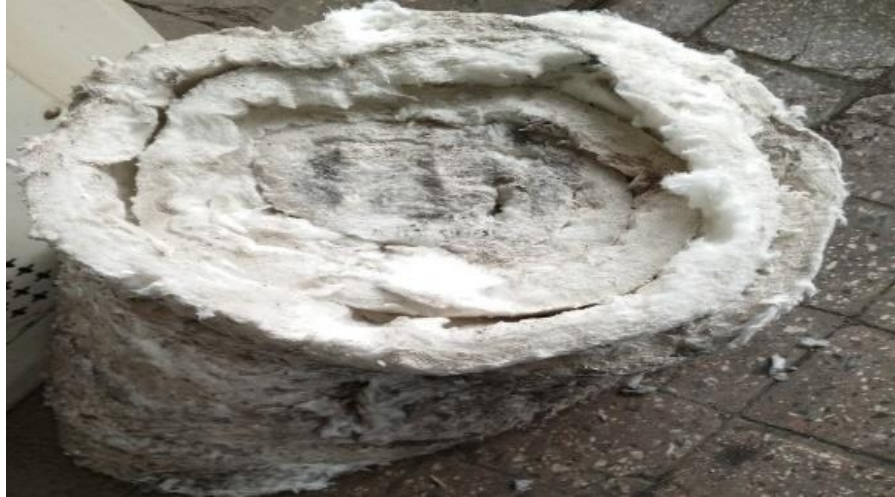
Figure 3.3 Asbestos for thermal insulation
