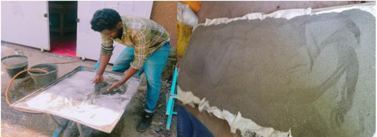
Appendix D1: Pictures taken during preparation of saturated surface dry sample for fine aggregate test.
