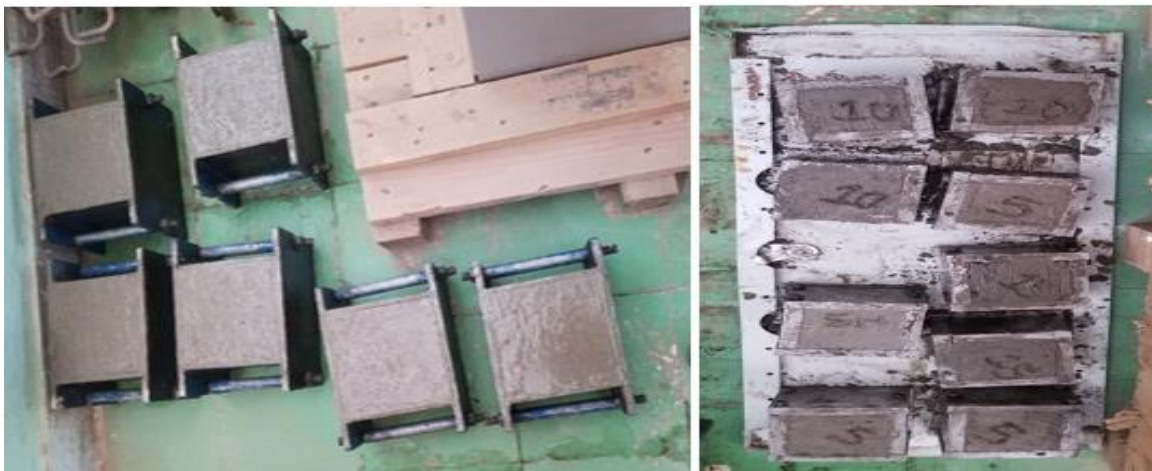
Appendix D7: Pictures shows casted samples: (150*150*150) mm sized cube for compressive strength test and (70*70*70) mm sized cube for water absorption test.
