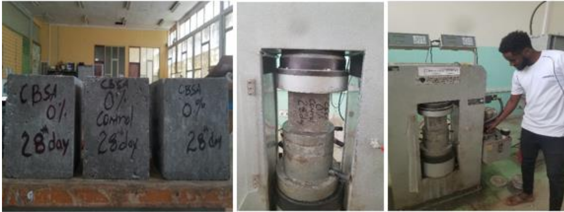
Appendix D9: Pictures shows sample preparation for compressive test and during conducting the test.
