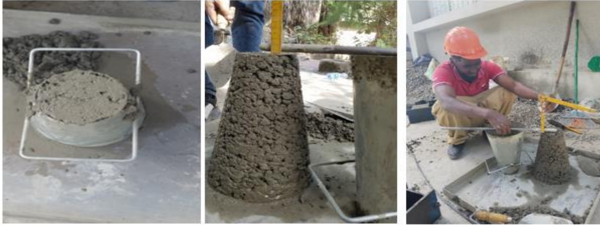
Appendix D6: Pictures captured during slump test.
