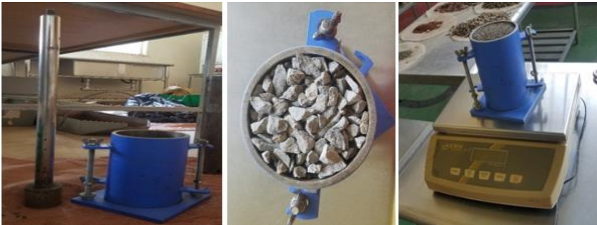
Appendix D4: Pictures captured during conducting unit weight test for fine aggregate and coarse aggregate.
