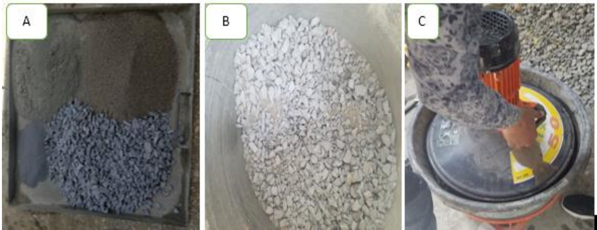
Figure 3.6: Pictures shows batching and mixing procedure: A) batched ingredients, B) dry mixing, and C) wet mixing:.
