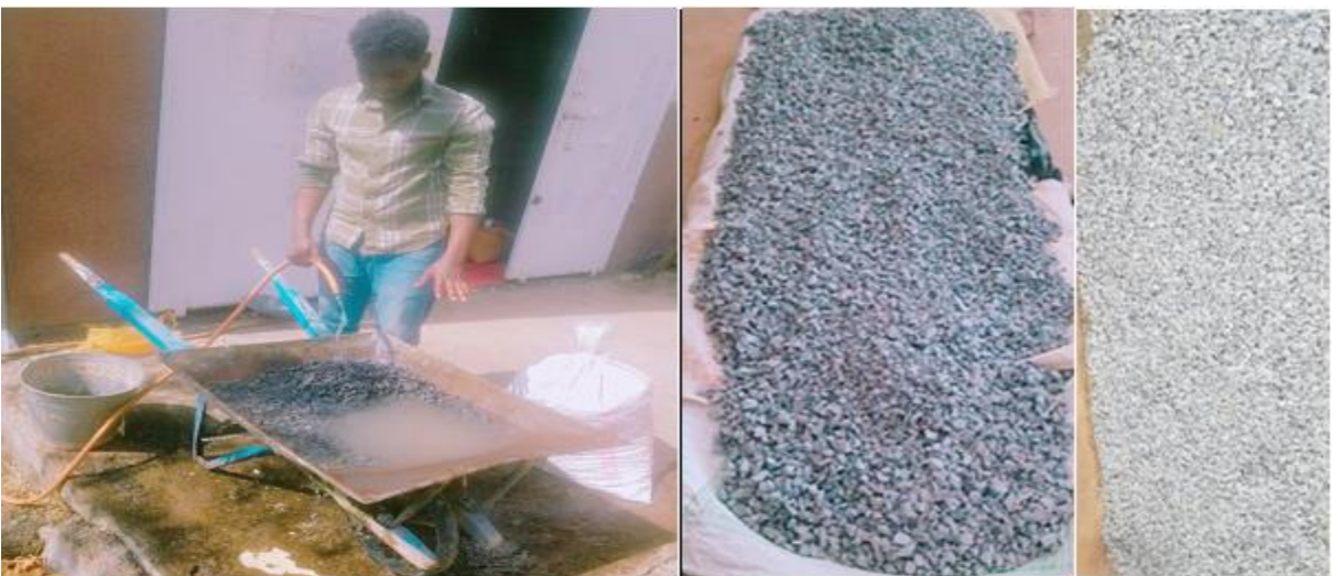
Appendix D2: Pictures taken during fine and coarse aggregate washing and drying.
