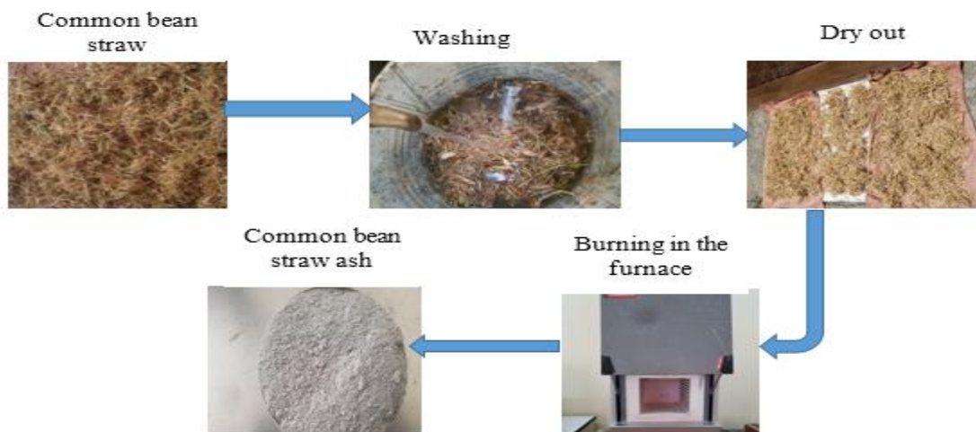
Figure 3.4: The process of common bean straw ash preparation.
