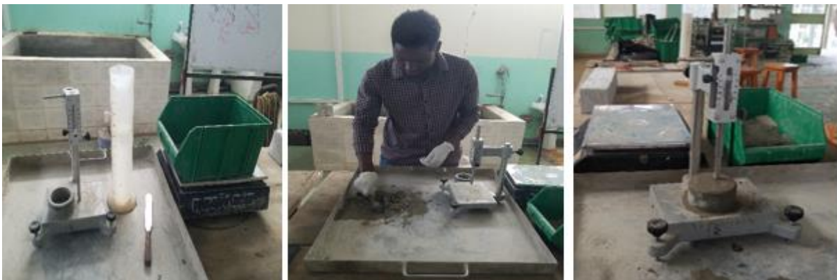
Appendix D5: Picture taken during normal consistency and setting time test.
