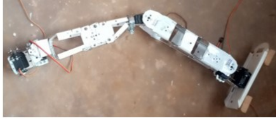
Figure 5.1: Dinkinesh Biped humanoid hardware right leg configuration and assembly.
