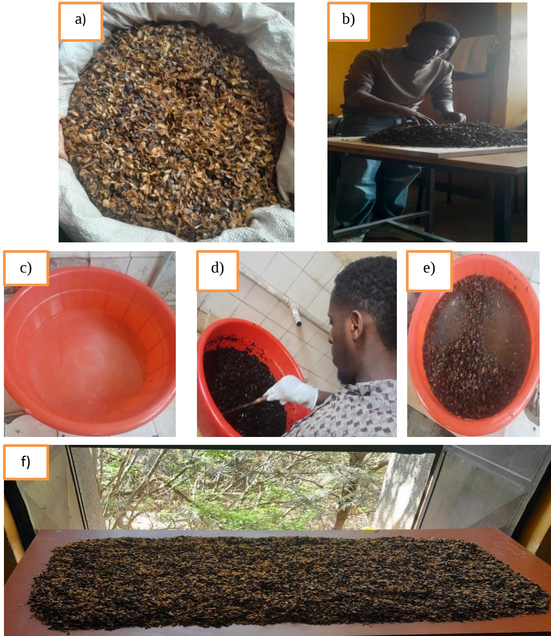
Figure 3.9 Coffee husk treatment: (a) Raw CH (b) Manual cleaning of CH (c) Mixture of distilled water with NaOH (d) CH treated with NaOH (e) Dried CH after treatment
