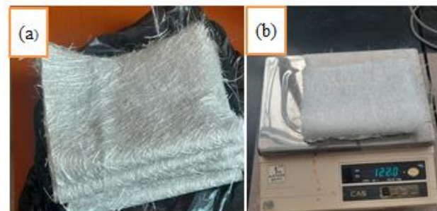
Figure 3.2 (a) Chopped E-glass fiber (b) E-glass fiber measurement
