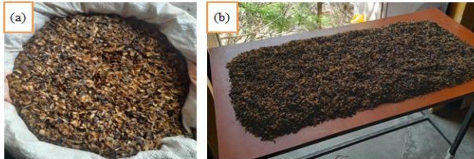
Figure 3.4 (a) Untreated coffee husk (b) Treated coffee husk
