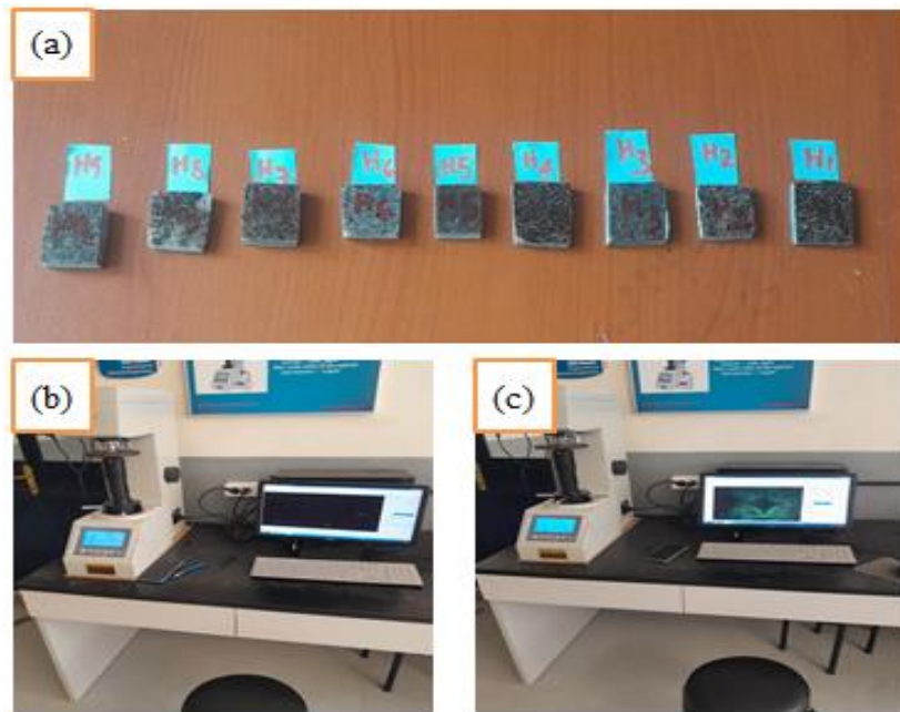
Figure 3.21 Hardness testing: (a) Specimens for hardness testing (b) Vickers hardness machine (c) Adjusted specimen
