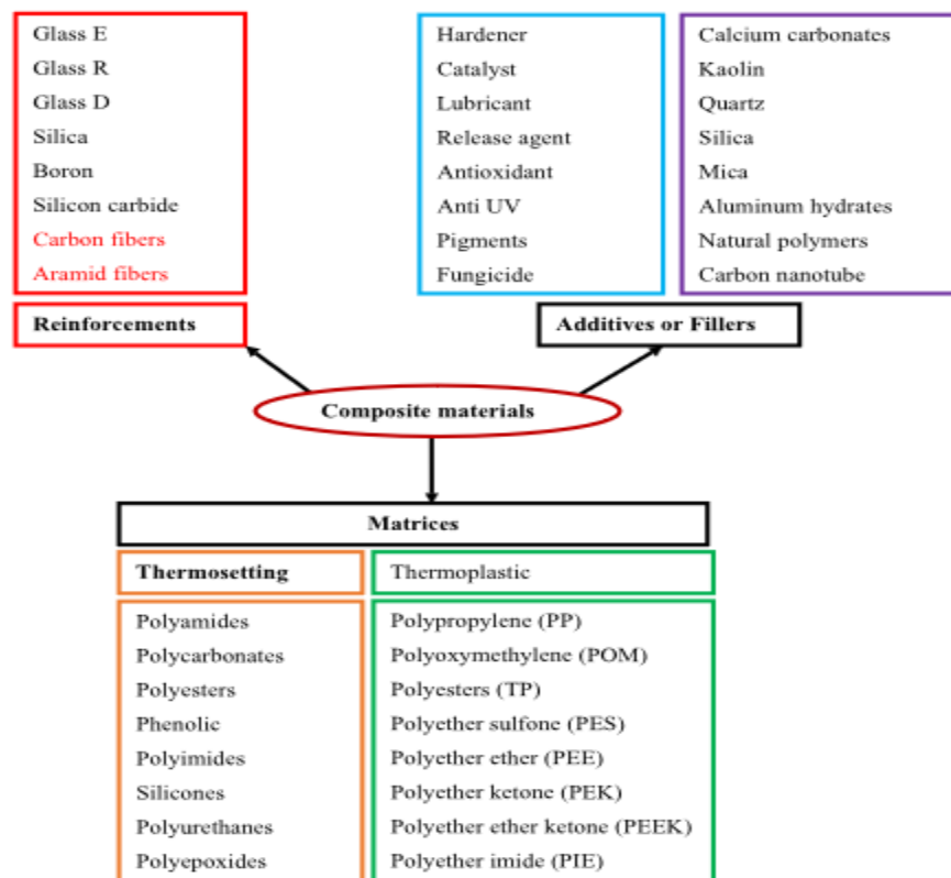
Figure 1.1 Polymer matrix composite formulation (Hsissou et al., 2021)
