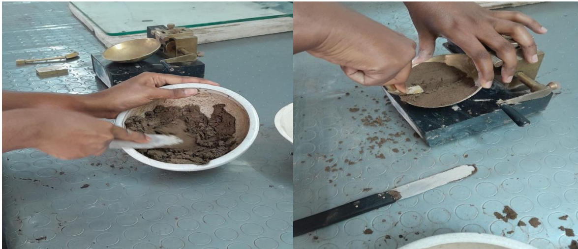
FIGURE 3.6: ATTERBERG LIMITS TEST
