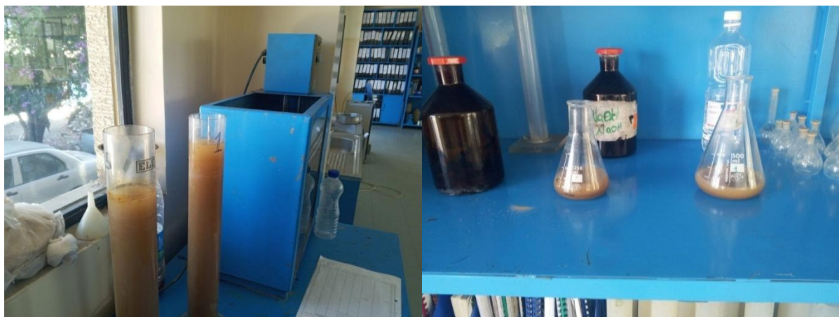
FIGURE 3.13: DOUBLE HYDROMETER TEST
