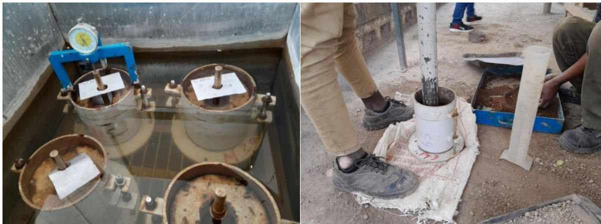
FIGURE 3.8: SPECIMEN PREPARATION AND SOAKING FOR CBR TEST
