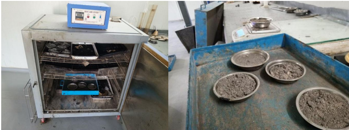
FIGURE 3.5: NATURAL MOISTURE CONTENT DETERMINATION
