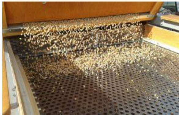
Figure 2.2. Mechanical seed cleaner
