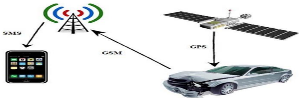
Fig 2. 6 GSM and GPS based Accident detection Mechanism (Zhang et al., 2010)
