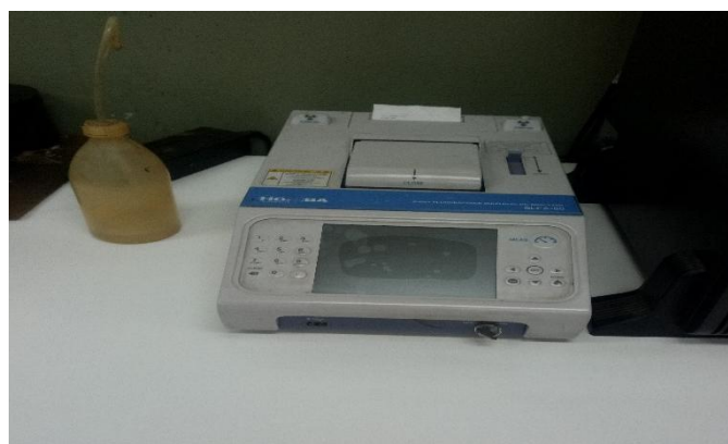
Fig. 28: Apparatus for determination of total sulfur, %wt
