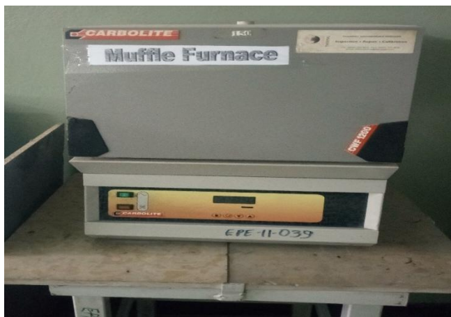
Fig. 25: Apparatus for determination of ash content
