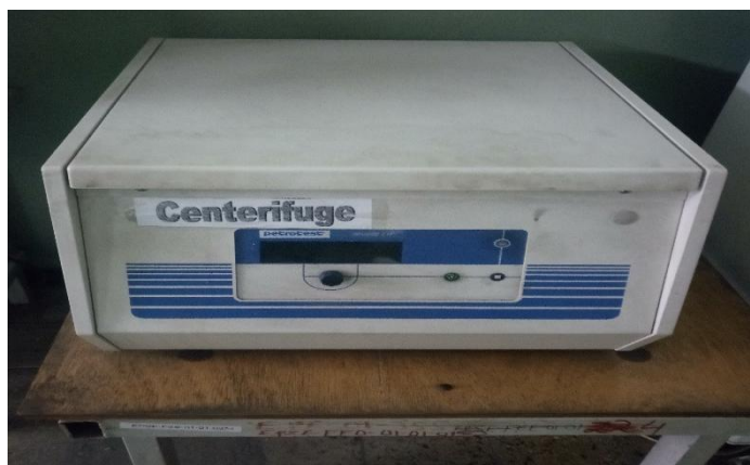
Fig. 26: Apparatus for determination of water and sediment, V/V %
