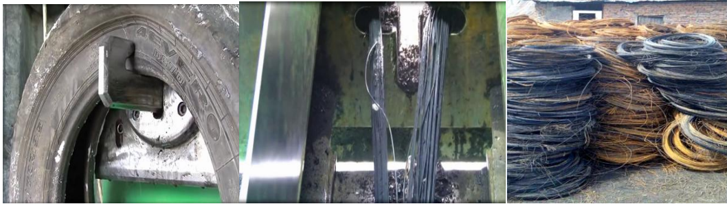
Fig. 13: Hang wa steel wire remover and its process
