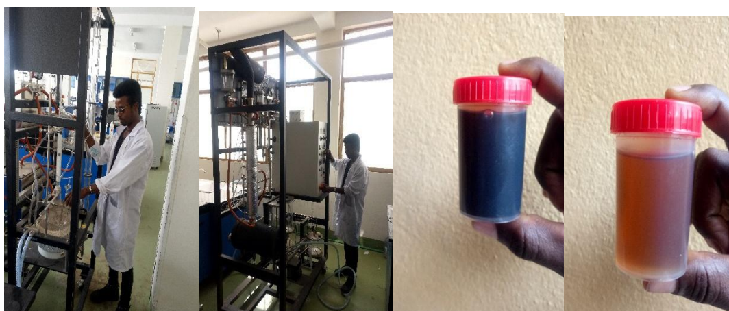
a) Distillation process b) crude tyre oil c) diesel tyre oil
