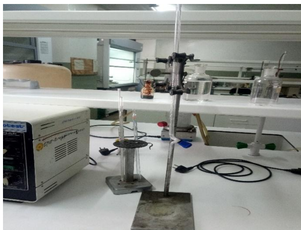
Fig. 27: Apparatus for determination of total acidity, mg KOH/g
