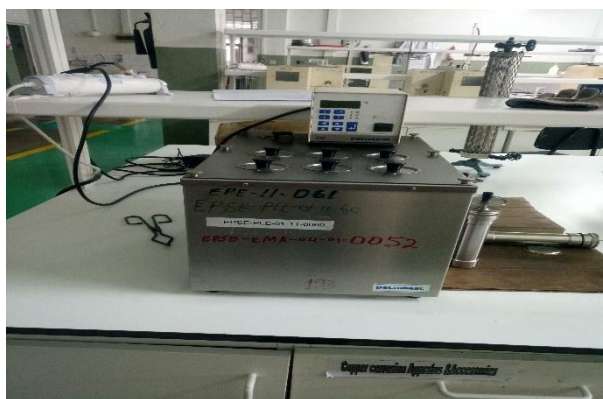
Fig. 23: Apparatus for determination of corrosion strip corrosion 3hrs @100 0 C.
