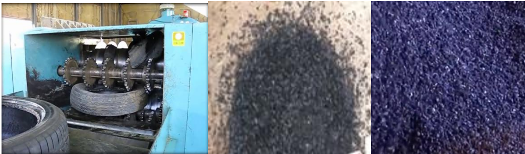
Fig. 14: Hang wa scrap tyre shredder and shredded tyres
