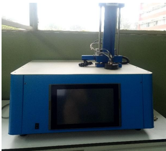
Fig. 22: Apparatus measuring cloud point
