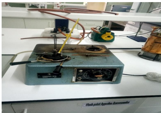
Fig. 21: Apparatus for determination of flash point
