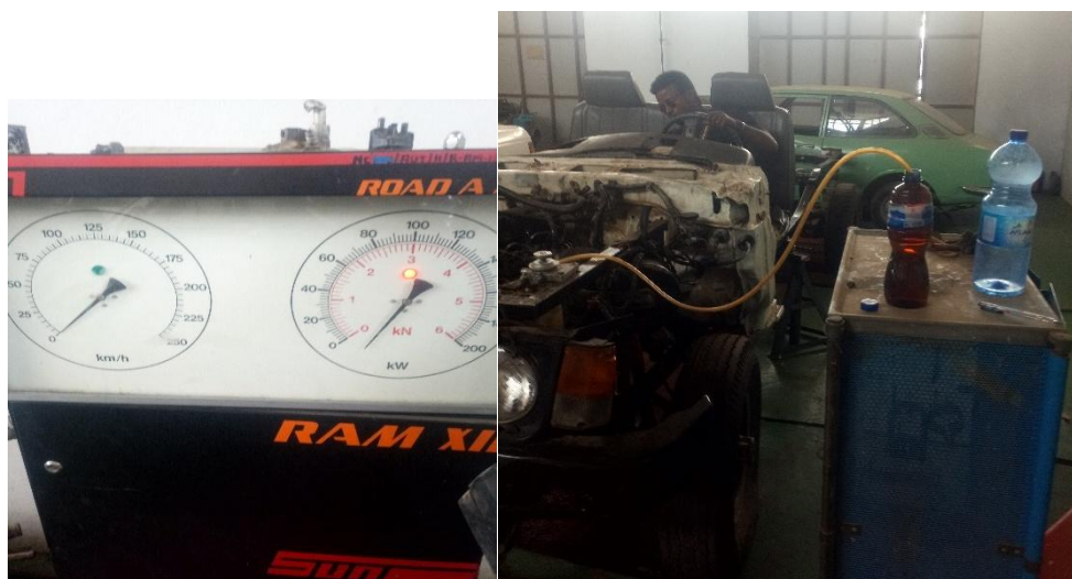
Fig. 30: Chassis dynamometer for vehicle (engine) performance testing.
