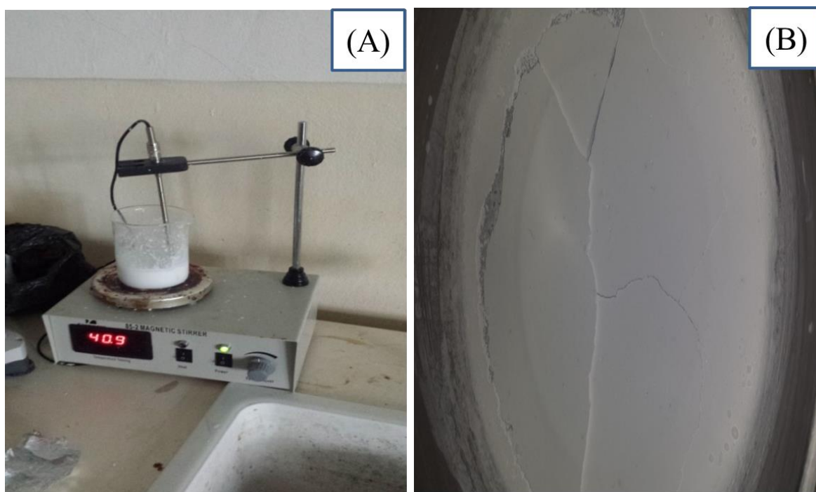
Figure 12: Impregnation process (A) Ca-Zn impregnation of catalyst and (B) Ca-Zn impregnation after drying in oven
