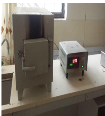
Calcination in Muffle furnace at various temperatures
