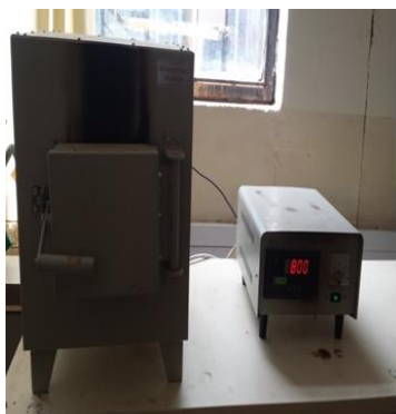
Calcination in Muffle furnace at various temperatures
