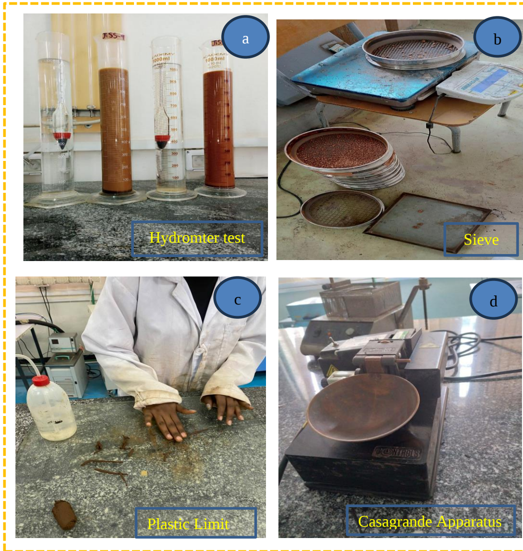
Figure 3. 4: (a) hydrometer (b) Sieve (c) Plastic limit (d) casagrande apparatus tests of soils
