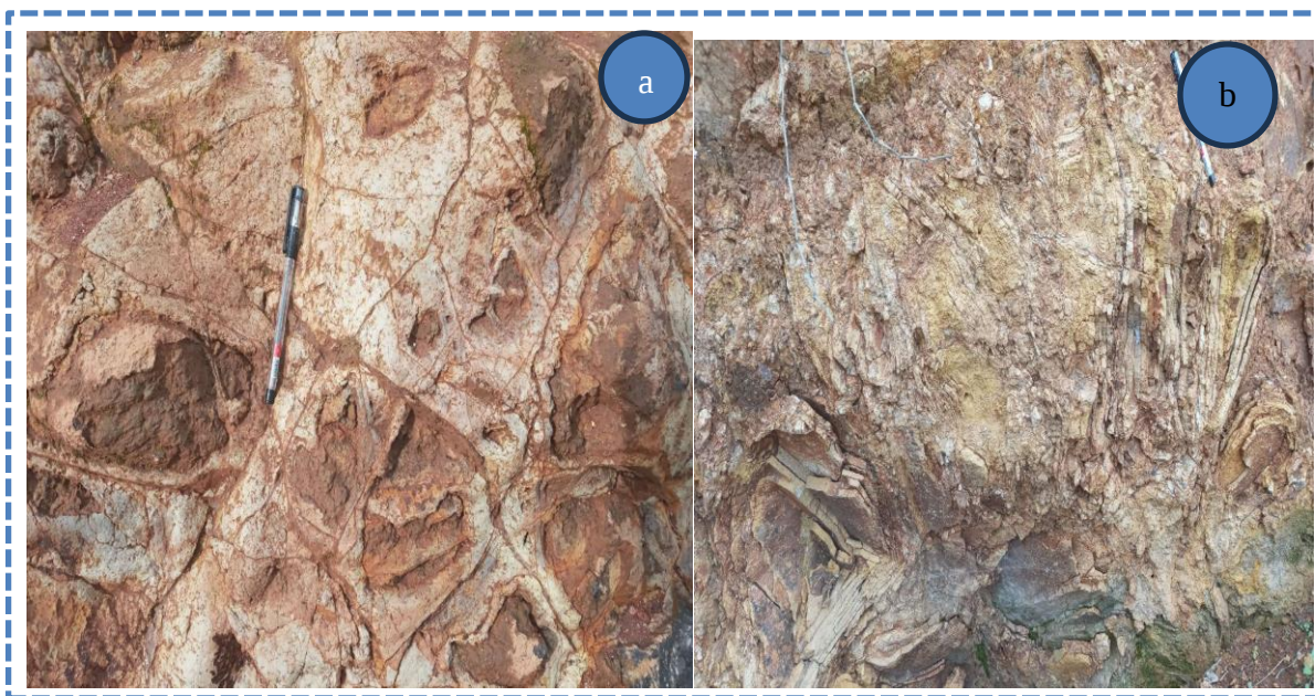
Figure 4.7 (a) Onion (exfoliation) weathering and (b) burst (spheroidal) weathering
