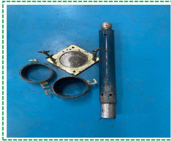
Figure 3. 7: Equipment used for compaction test
