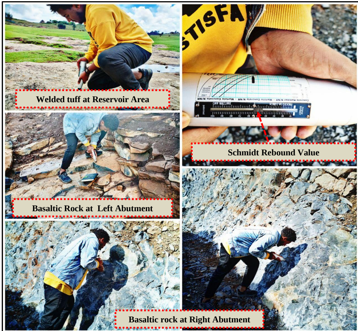
Figure 3.2. In-situ rock strength estimation test using Schmidt hammer.
