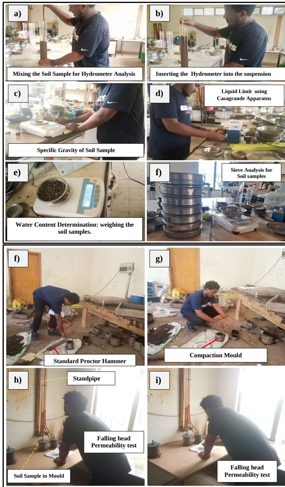
Figure 3.3. Soil laboratory tests (water content, specific gravity test, grain size analysis (sieve and hydrometer analysis), Atterberg limit test, compaction test, falling head permeability.)
