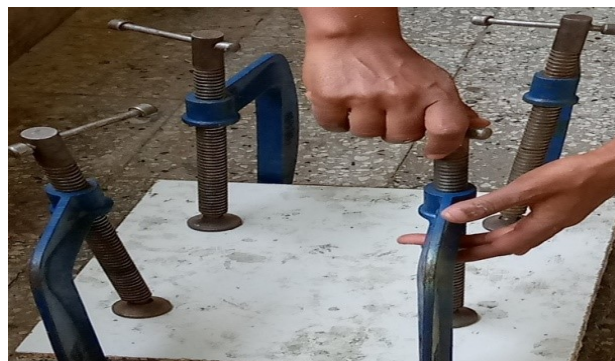
Figure 3.7 Fabrications of Composites with Tightening by C-clamp
