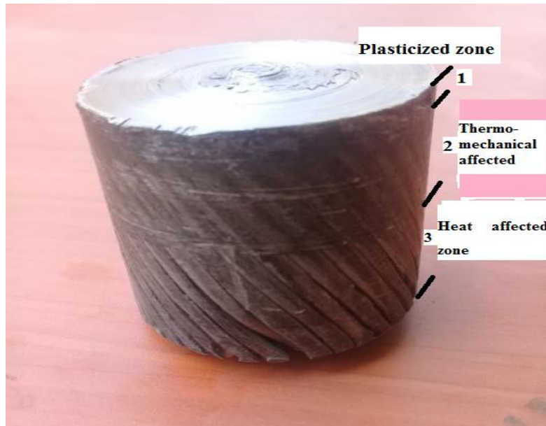
Figure 4. 3 Friction consolidated wire disc with three different zones
