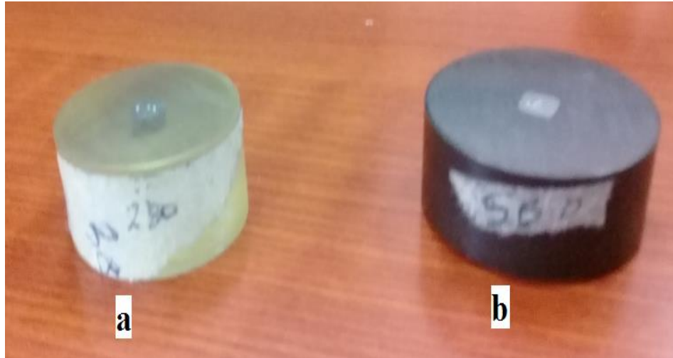
Figure 3. 10 Samples mounting: a) Cold mount, b) Hot mount
