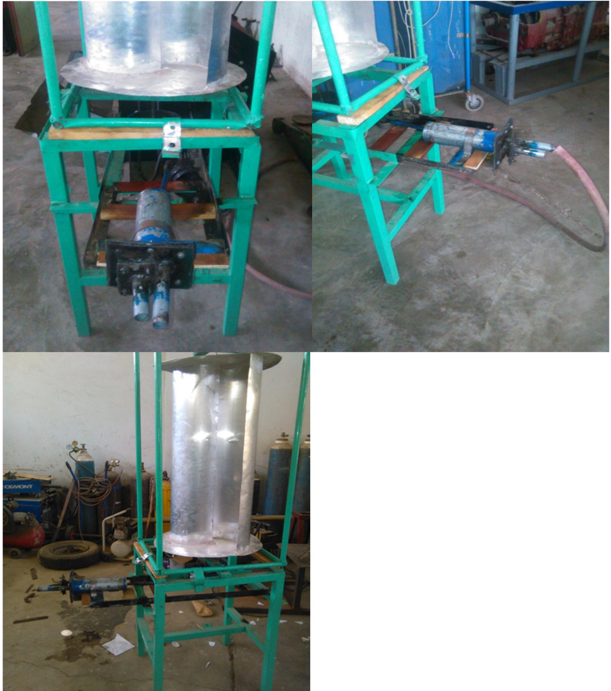
The prototype of the piston pump with wind turbine assemble
