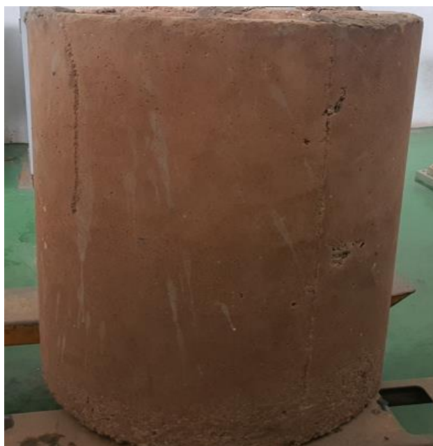
Figure 5-2: Fabricated refractory material.
