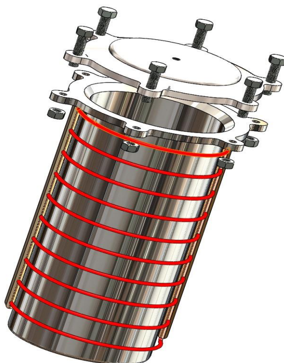
Figure 4-3: Model of reactor assembly.
