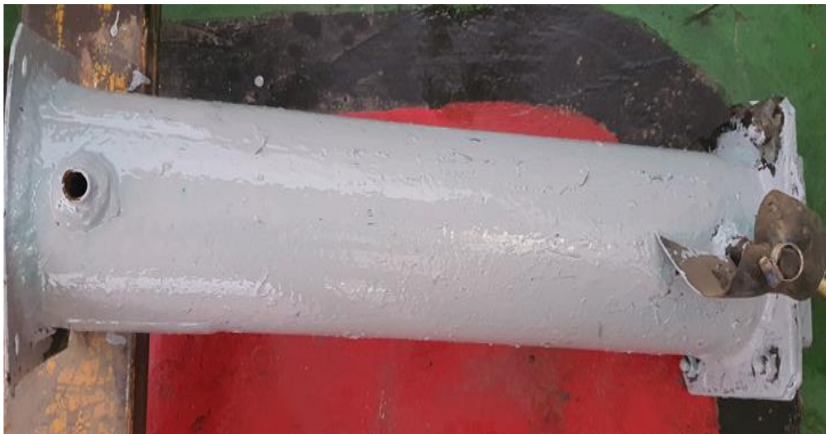
Figure 5-3: Constructed condenser system.
