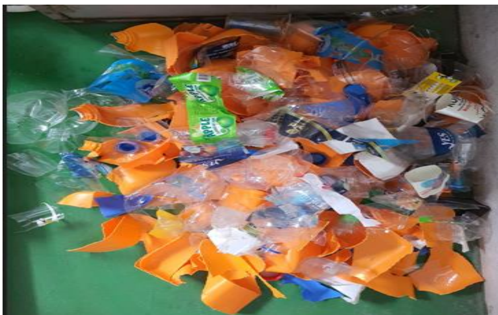
Figure 5-5: Shredded waste plastic for pyrolysis.
