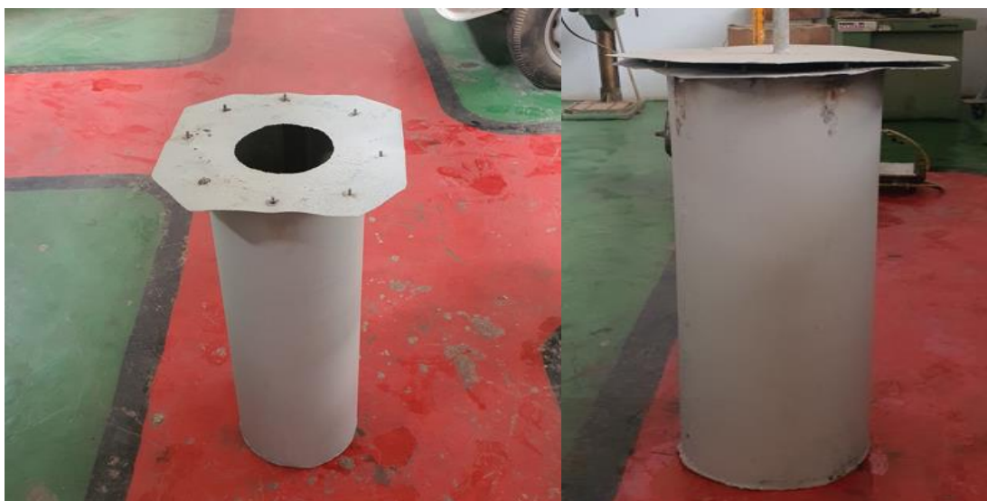
Figure 5-1: The pyrolysis reactor with flange.
