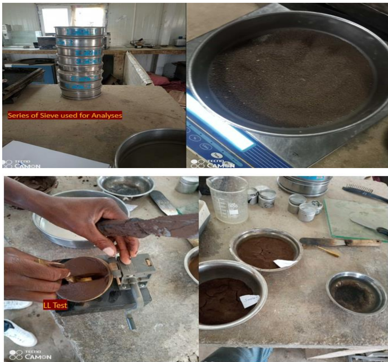
Figure 3-10 Sieve analyses and Atterberg limit tests of soils
