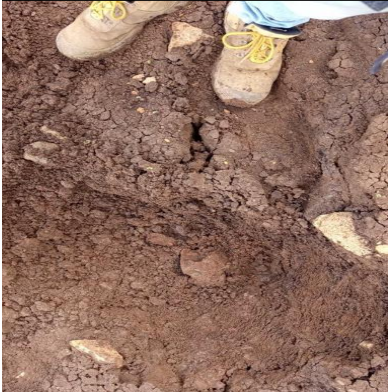
Figure 3-8 Pit Depth 1m for sample taken to Laboratory tests at 11+820
