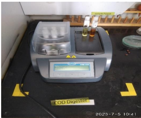
COD digester (measuring COD)
