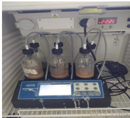
BOD digester (BOD measurement)
