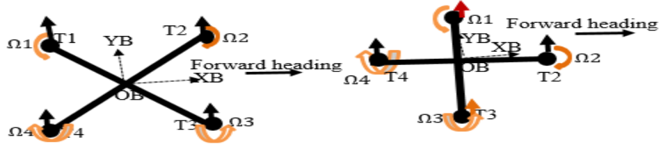
Figure 3.5 pitch movement of quad-rotor
