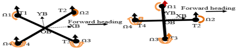
Figure 3.4 Roll motion of quad-rotor for cross and plus configuration
