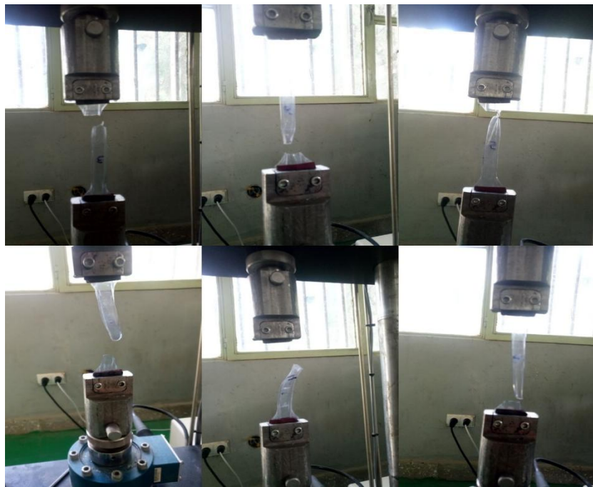
Figure 4. 1. Samples after plastic failure on UTM during tensile testing
