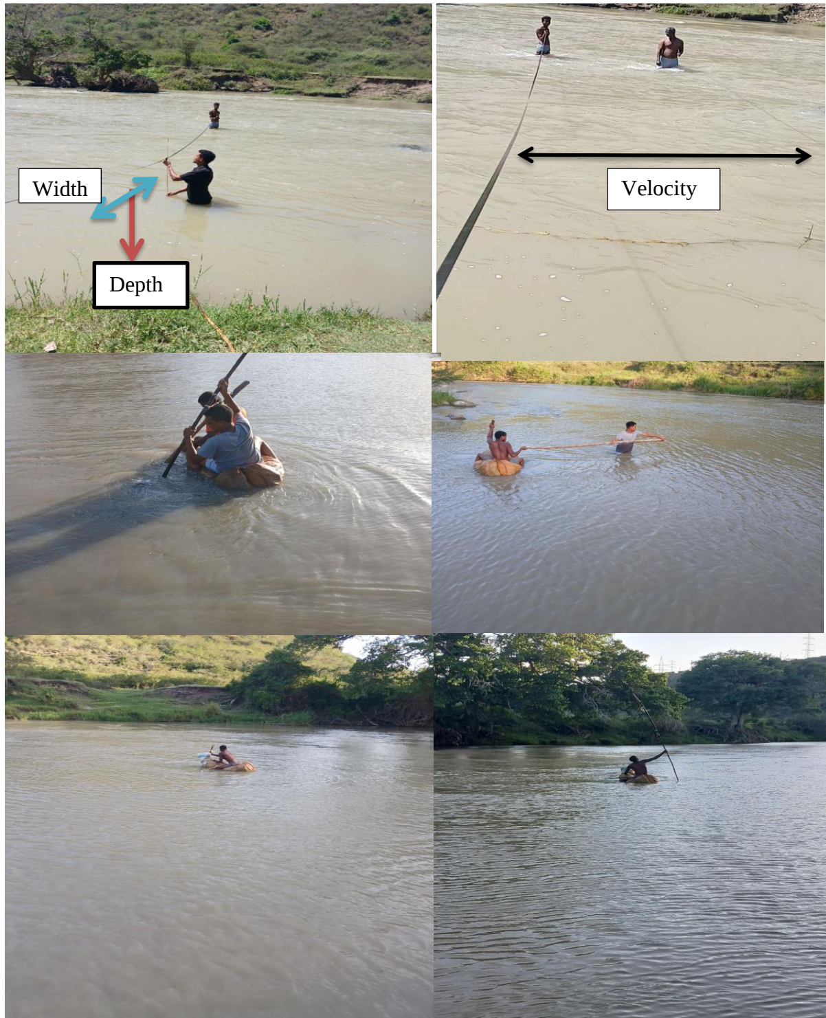
Figure 3.4 the cross section and velocity measurement of the river at sites
