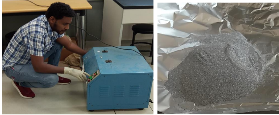
Figure 3.3 (a). High energy ball milling machine for powder mixing process and (b) the final milled powder mixture of the AlMg-SiC composites.
