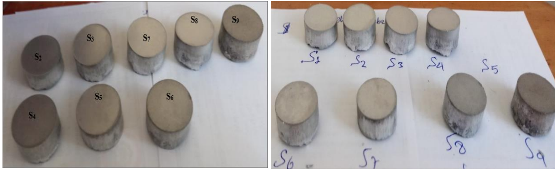
Figure 3.6. The AlMg-matrix (S 1 , S 2 , S 3 ) and AlMg/SiC composite samples (S 4 -to-S 9 ).
