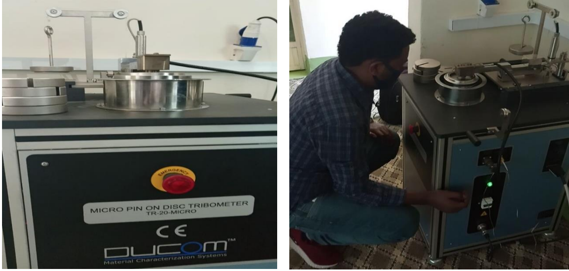
Figure 3.14. Pin-on-disc (DUCOM TR-20 MICRO) equipment and testing
