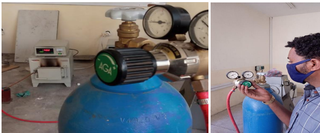
Figure 3.5. Experimental set up for sintering the green compacted samples in the furnace.
