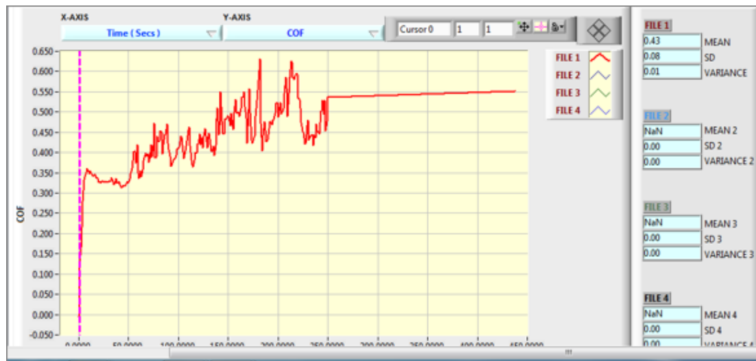
Figure B-2. (COF) Vs time for AlMg-5%SiC composite samples (S4, S5 and S6).
