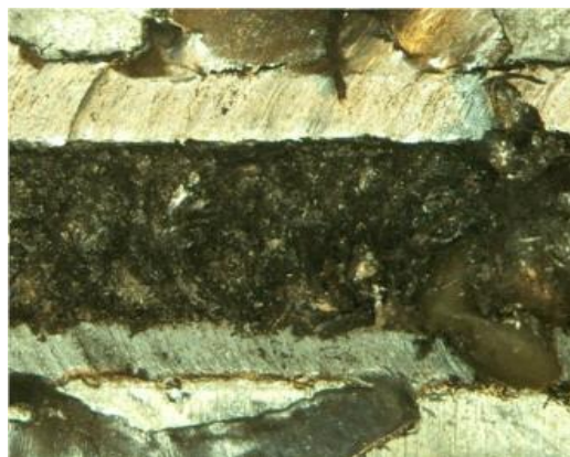
Microstructure observation of joint 3 i.e. 850 RPM, 63 mm/min
