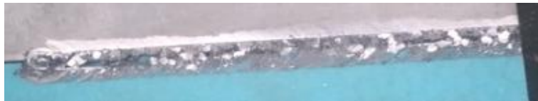
Figure 4. 2 Joints formed by 850RPM and 40mm/min
