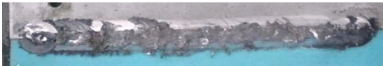
Figure 4. 4 Joint formed by 850RPM and 63mm/min
