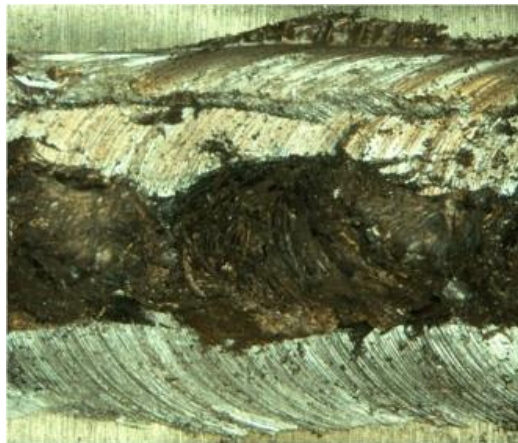
Microstructure observation of joint 2 i.e. 850 RPM, 50 mm/min, 2.5^0
