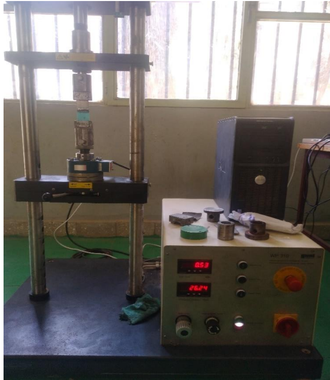
Figure 3. 17 machine setup for tensile test
