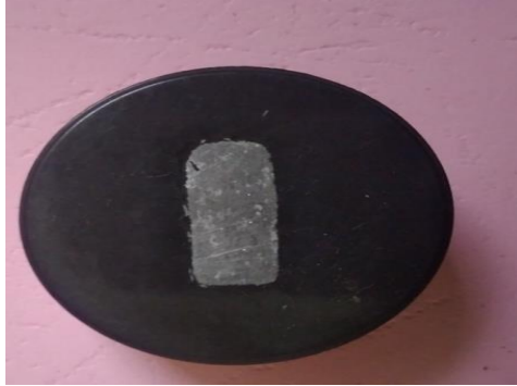
Figure 3. 13 Sample cut Al alloy for hardness test
