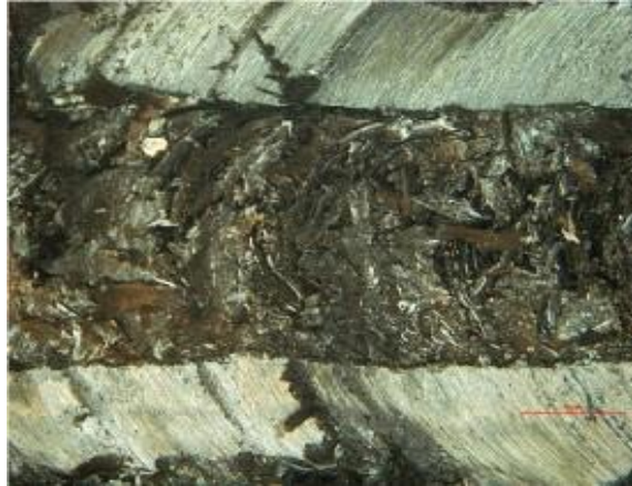
Microstructure observation of joint 4 i.e 1000 RPM, 40 mm/min, 2.5^{\circ}
