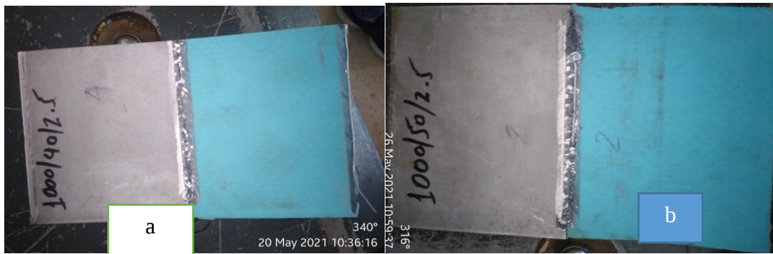
Figure 3. 9 FSW joints mad by a) 100RPM and 40mm/min b)1000RPM and 50mm/min
