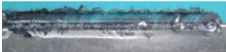
Figure 4. 3 Joints formed by 850RPM and 50mm/min
