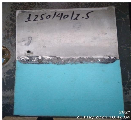
Figure 3. 10 FSW joint made by 1250RPM and 40 mm/min
