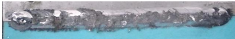
Figure 4. 10 Joint formed by 1250RPM and 63mm/min
