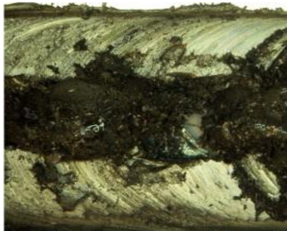
Microstructure observation of joint 6 i.e. 1000 RPM, 63mm/min 2.5^{\circ}
