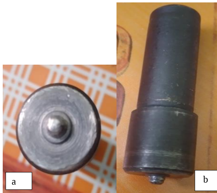
Figure 4. 1 a) Bottom view FSW tool after welding b) Front view of FSW tool after welding.
