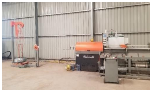
a) Wire straightening machine
