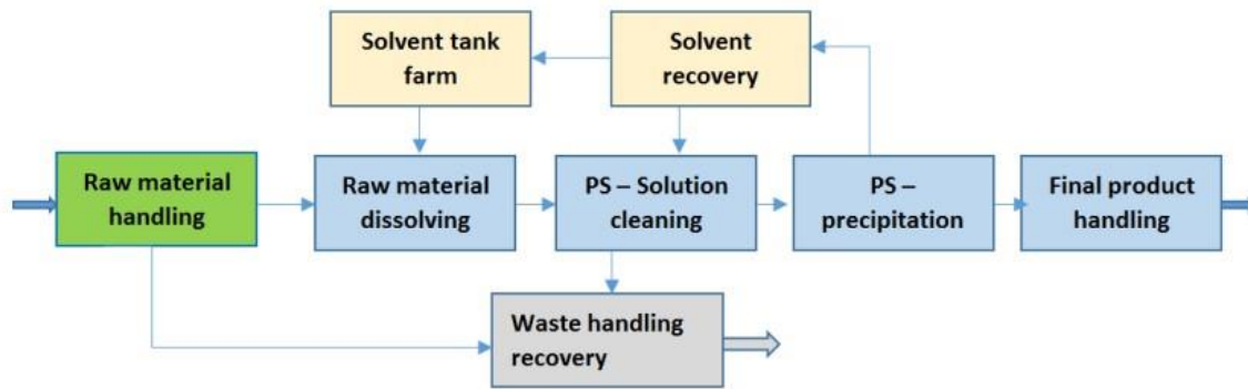
FIGURE 2.10 Recycling Process of EPS Materials (Nyambara et al., 2017)
