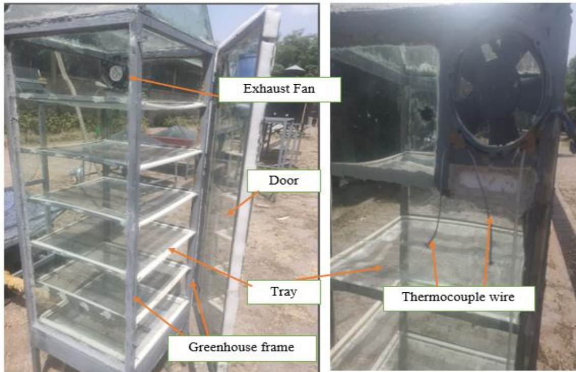
Figure 5. 4: Construction of the greenhouse
