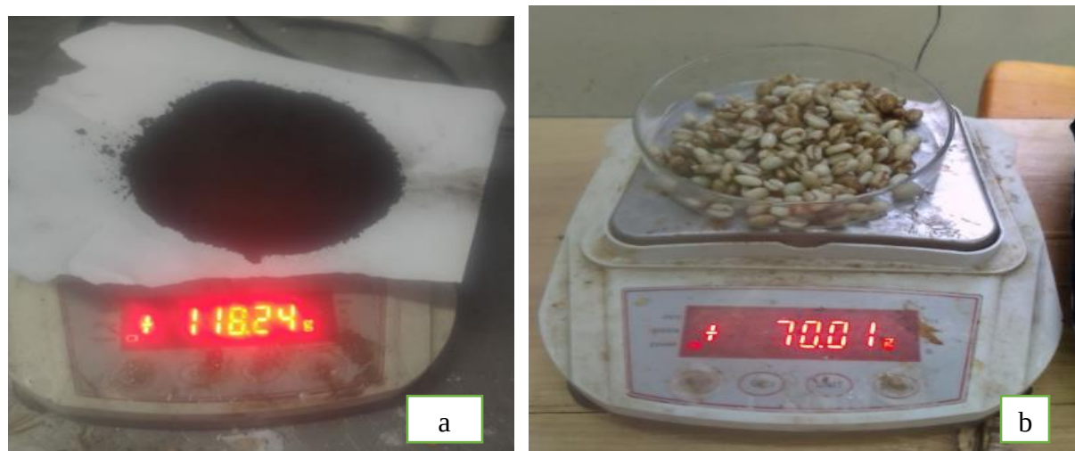
Figure 5. 9 : Digital weight balance during measurement a) measuring mass of copper oxide b) measuring mass of coffee beans
