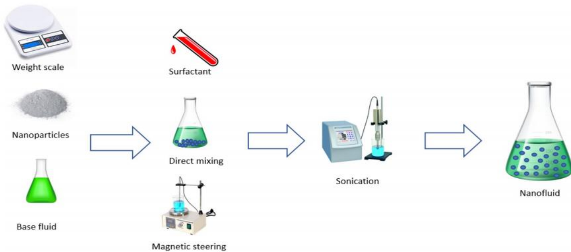
Figure 5. 10: Preparation procedure of nanofluids in laboratory (Abu and Bodius, 2020)
