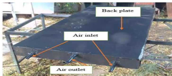
Figure 5. 3: view of solar collector from bottom direction
