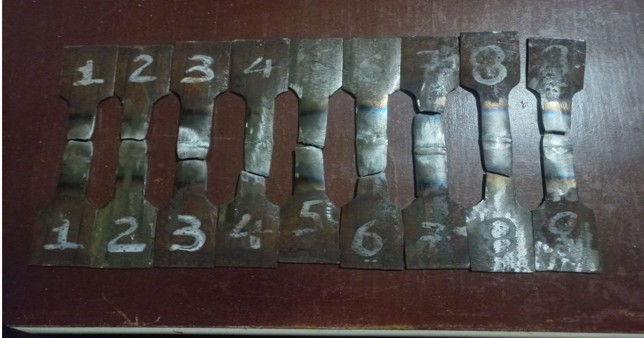
Figure 3.8 the result after tensile test at FDRE Technical and Vocational Training Institute.
