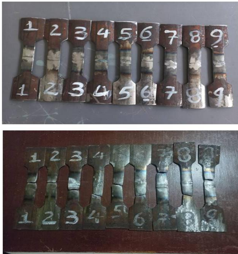
Figure 4.5 Tensile test samples prepared before testing and after testing
