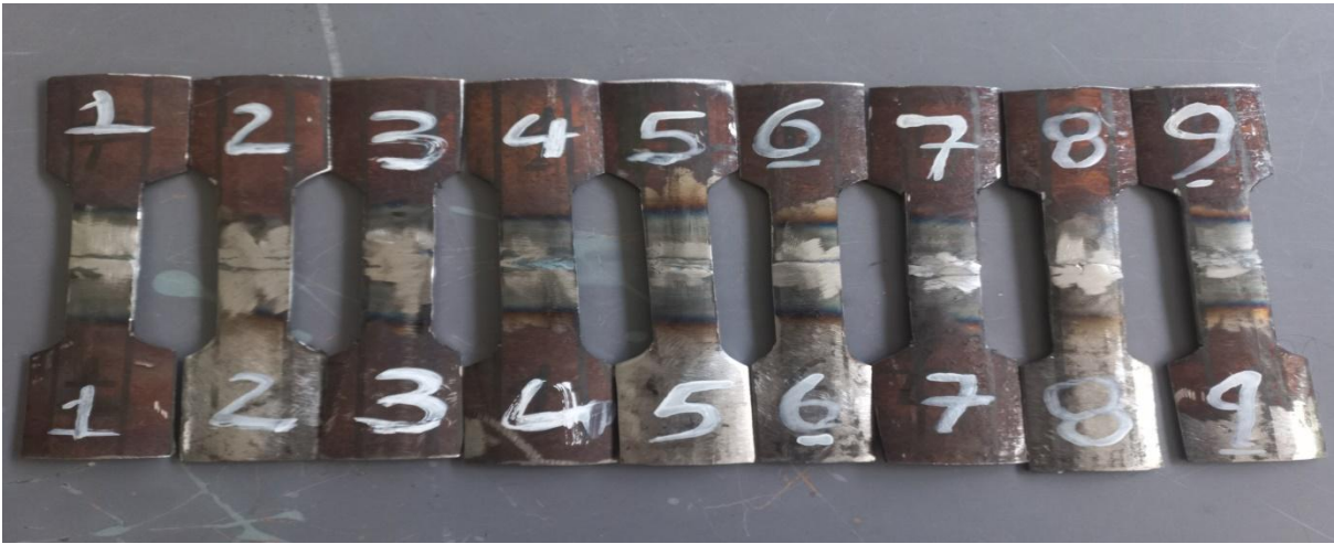
Figure 3.6 sample prepared for tensile strength from mild steel specimens
