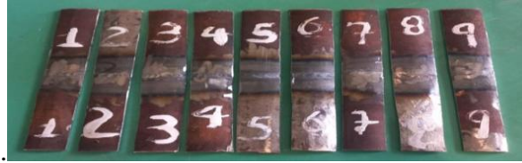
Figure 4.2 Hardness sample prepared for test.
