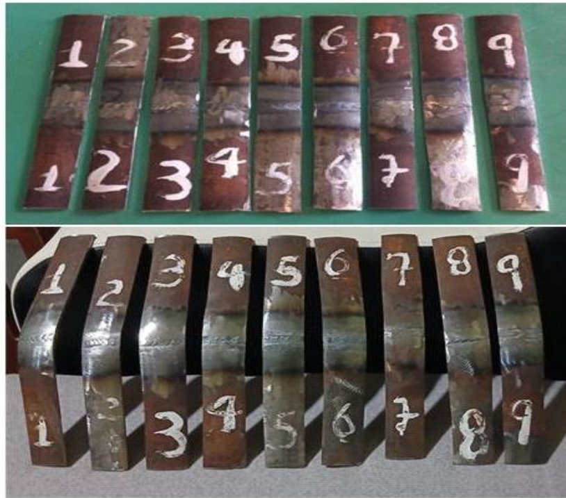
Figure 4.7 Bending test specimens, showcasing their preparation before testing and their condition after testing
