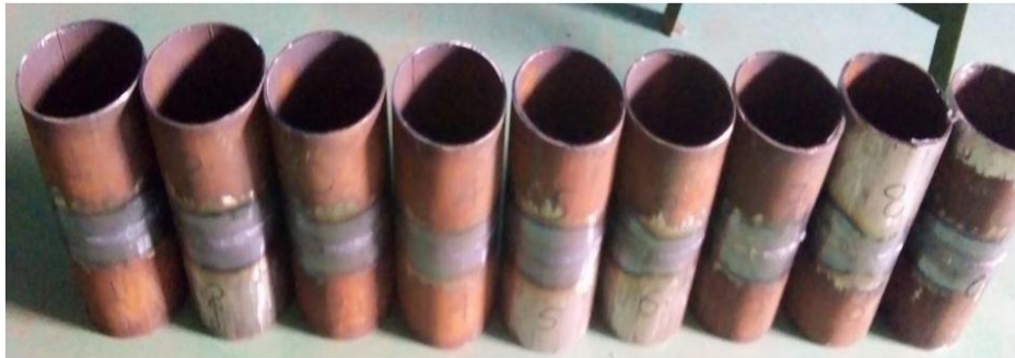
Figure 4.1 Illustrates the welding experimental work carried out in this investigation, showcasing the welded specimens in order
