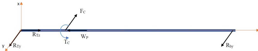
Figure 4-39 FBD of Idler Shaft
