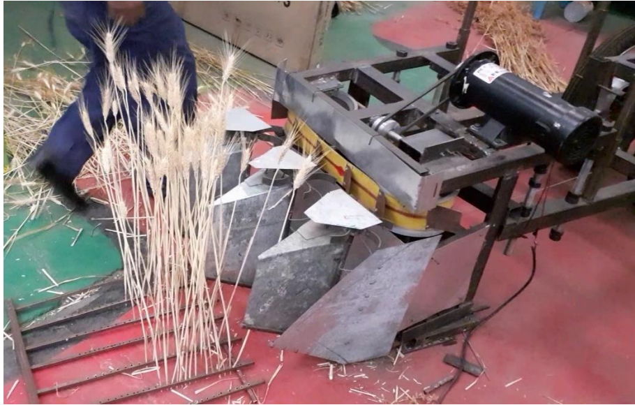
Photo 4-8 Quadruple Rows of Straws before Cutting
