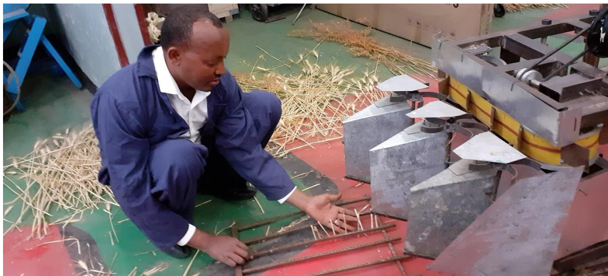
Photo 4-3 Single Row of Straws after Cutting
