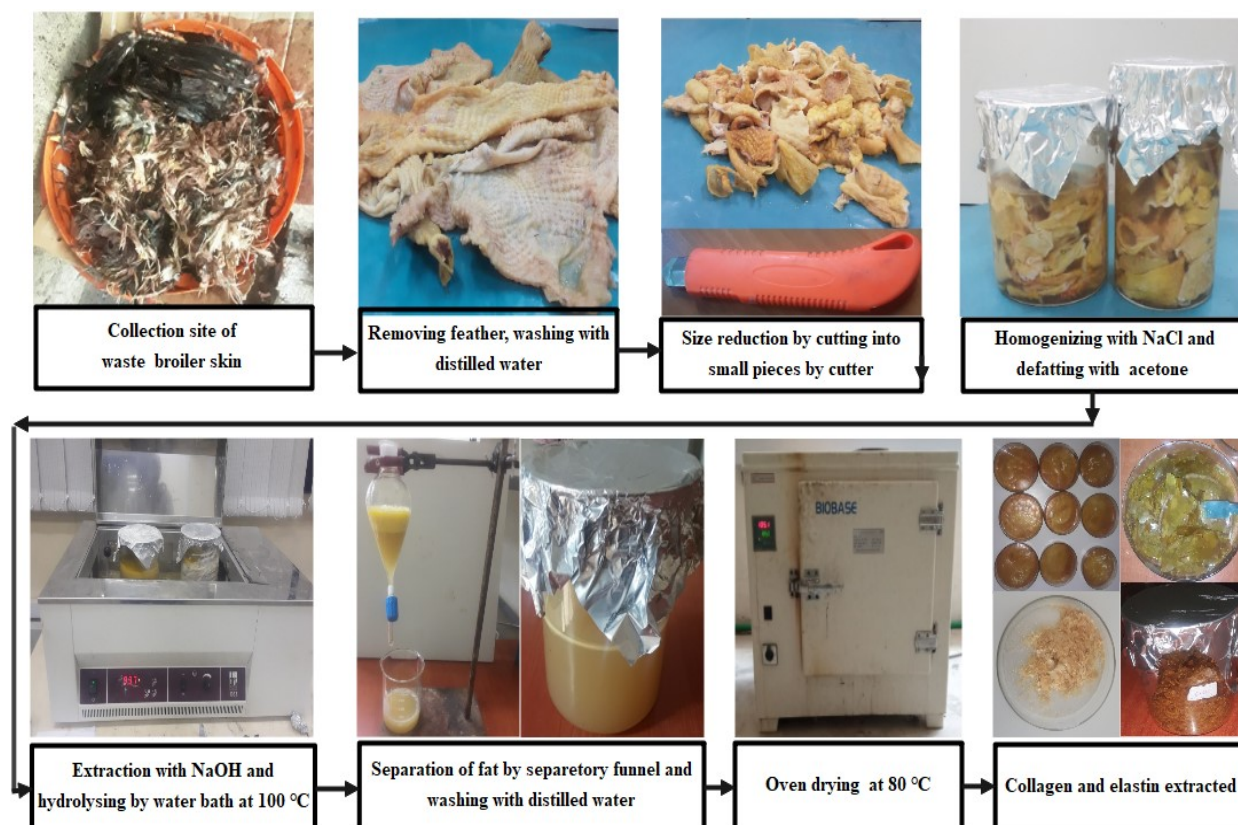
Figure 3 - 4: Process flow for extraction of COL/ELS from broiler skin.
